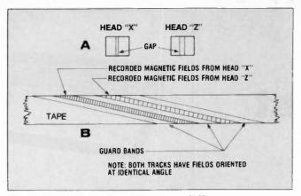
Fig. 1 – Vertical orientation of head gaps (1A) necessitates guard bands (1B) between recorded tracks to eliminate crosstalk.
