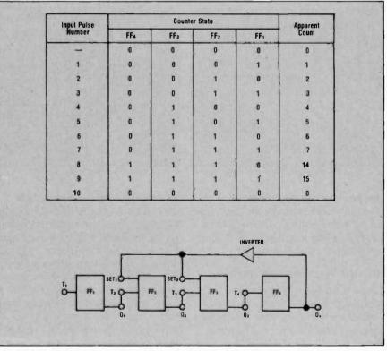
Fig 6-Block diagram of a scale of 10 counter and the table showing its summary of states.
