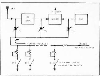
Fig. 2-A basic push-button channel selection system.
