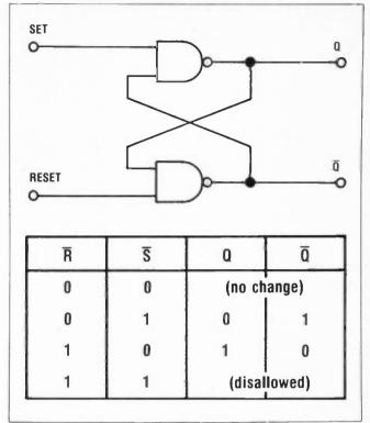
Fig 2-Two input NAND gate flip-flop with its associated truth table.
