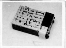
the chart section can also serve as a direct current reader to 10mV/cm. The design format includes: automatic start
