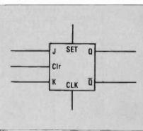
Fig 4-Block diagram of a J-K flip-flop
