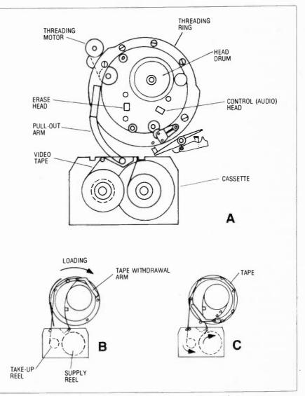
Fig. 3 – Progressive views of the tape threading operation. Figure 3A shows tape position at the start; 3B is a view of the half completed threading operation; and 3C shows the completed threading.
