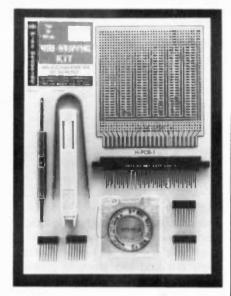
WSU-30, wraps and unwraps 30 AWG wire on .025 square pins and strips the wire. The board features glass coated epoxy laminate construction with solder coated 1 oz. copper pads. Sockets have gold plated terminals and thermoplastic bodies. The wire dispenser includes 50 feet of kynar insulated, silver plated copper wire. The kit is priced at \$25.99.
