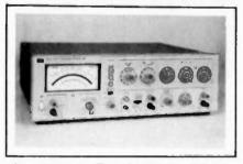
nine ranges. The fundamental frequency range for distortion measurements is from 10 Hz to 110 kHz; harmonics are indicated up to 330 kHz. As a true-rms calibrated voltmeter, Model 339A measures input levels from 1.0 mV RMS to 300 V RMS full scale over a frequency range from 10 Hz to 110 kHz. As an ultra-low distortion oscillator, it delivers sinusoidal frequencies from 10 Hz to 110 kHz with output level adjustable from 1mV to 3V rms into a 600 ohm load. Priced at \$1900.
