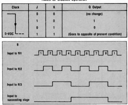
Fig 5-Timing diagram for three plus stage flip-flop circuit showing input and output wave forms.
