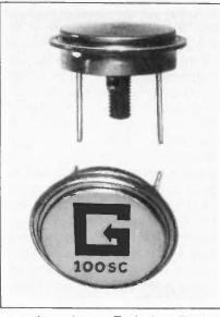
operating voltages. Typical applications are in inverters, switching regulators, power amplifiers and similar high current circuits. Being based on Germanium technology, the GPD 100SC series also is said to give high gain (HFE = 120 typical at -60A IC, -1V VCE), high efficiency, low input voltage and, above all, very low saturation voltage.
