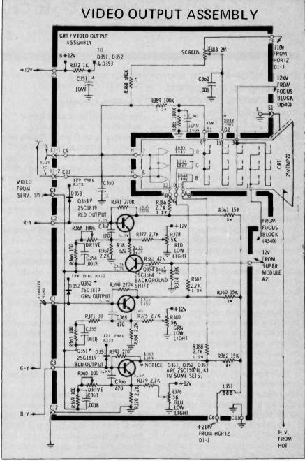
Figure 7 The video output assembly
