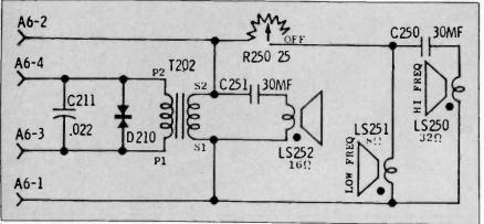
Figure 4 The "Audio Spectrum" sound circuitry
