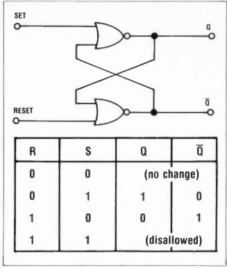
Fig 1-Two input NOR gate RS flip-flop with its associated truth table.
