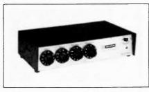
mixing, normally found only in expensive consoles, for nearly zero interaction among its four input controls. Active mixing is said to minimize the residual mixing bus noise and provides constant preamplifier gain as more input channels are added. The CSM has four microphone inputs, two of which are convertible to auxiliary inputs. Each input can accept either high- or lowimpedance microphones. Suggested list price is \$137.25.
