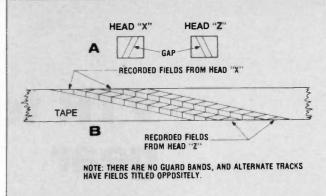
Fig. 2 – Oppositely slanted head gaps (2A) permit recording with oppositely polarized tracks (2B) which in turn reduce crosstalk action without the use of guard bands.
