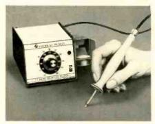
transformer and grounded soldering tip. The handpiece of the iron is lightweight with a four-foot super-flexible, oil-resistant cord. Heating element is built into the soldering tip, close to the point, which is pure iron and pretinned. Two replacement tips are available: needle point and chisel. Both may be filed to special shapes by the user to fit the job.
