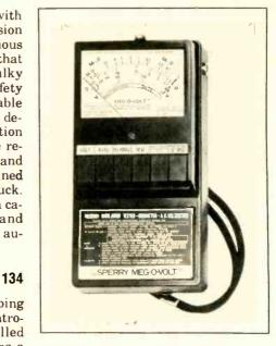
midscale, and the 520, which has a 1,000 megohm scale with a 20 megohm midscale. Both models have Rx1 and Rx100 resistance scales, as well as a 0-300 AC voltage scale. They feature keyboard push-button controls, threaded test leads, and a shock-resistant plastic housing. Powered by 8 AA batteries, the meter is portable. It develops a 500 VDC test voltage for insulation testing.
