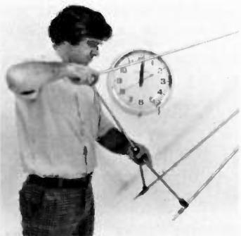
Tighten collar coupler, securing top radiator
