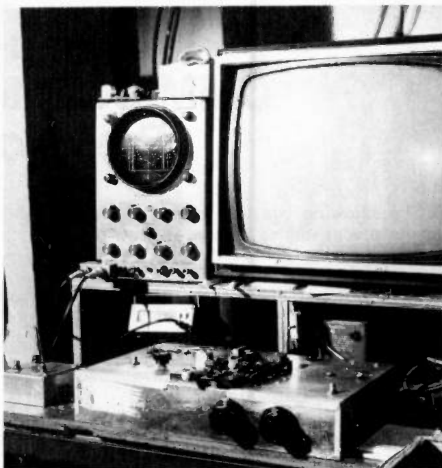
Modules are subjected to a vibration test while monitoring frequency and output as well as an air-check to uncover intermittents.
