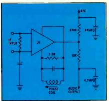
Fig. 8—Partial schematic of an FM detector using the ICQD. This circuit is identified as a quadrature detector by the presence of the 'phase coil" and not by the fact that an IC is
