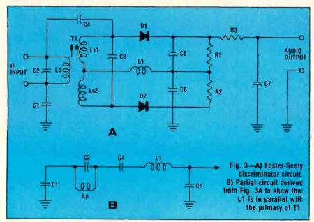
a great deal of pre-emphasis to the higher audio frequencies in an effort to improve the signal-to-noise ratio at the receiver end of the system. The receiver detector circuit includes a 75-microsecond RC deemphasis network which reestablishes the proper audio frequency response.
