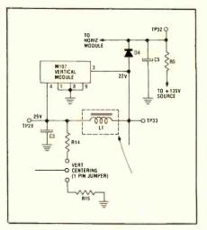
CAUSE: Partially shorted vertical output choke, L1 (Magnavox Part No. 320124-23). The resistance of L1 should be 9 to 10 ohms. A resistance reading of less than about 7 ohms indicates a possibly shorted choke. (The resistance of these chokes actually found to be partially shorted measured about 3 ohms.)
