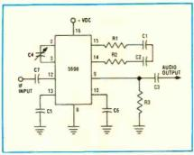
Fig. 10—Circuit of an FM detector equipped with the Signetics 560B IC PLL.
