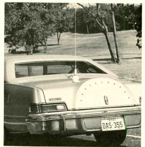
Fig. 6—This whip antenna from Breaker has a magnetic base encapsulated in ABS to prevent surface scratching. It is quickly removed for theft prevention.
