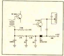
Fig. 3—Typical car radio automatic gain control (AGC) system. Defects in this system can cause audio distortion whose degree varies with received signal strength.
