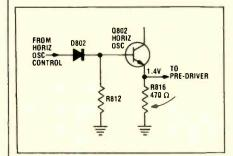
CAUSE: Slow stabilization of horizontal oscillator as result of increase in the value of resistor R816 (470 ohm, 10%, ½ watt). Replace R816 with Admiral Part No. 60A105-471 (470 ohm, 5%, ½ watt).
