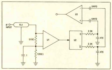
Fig. 11—Partial schematic of a pulse counting, or "digital," FM demodulator. This circuit uses a monostable multibrator and a pair of integrator networks to demodulate the FM signal. It is relatively independent of IF frequency and needs no alignment.
