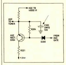
CAUSE: Defective capacitor C305 (5mfd, 50WVDC) in AGC circuit. If defect is verified, replace C305 with Admiral Part No. 67A200-509-7.
