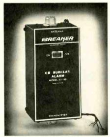
Fig. 5—A burglar alarm that is installed between a CB mobile unit and the antenna. When ground connection to either is broken, the alarm sounds.
