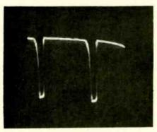
Fig. 3—Clipped horizontal sync waveform.
