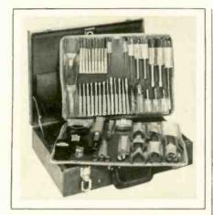
dividual tools, interchangeable screwdriver/nutdriver blades and handles, 10 ft. and 50 ft. measuring tapes, soldering iron, solder, and recharger. It has removable pallets in the lid and see-thru plastic tool pouches. Additional tool space is provided in the partitioned base.
