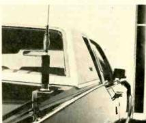
Figs. 10 & 11—Two somewhat similar antennaconcealment devices for CB that allow the user to lock the antenna inside the car trunk when not in use. Fig. 10 is the Stowit antenna from Holly Enterprises, and Fig. 11 is the Tuk-a-Way antenna from Deep South Marketing.
