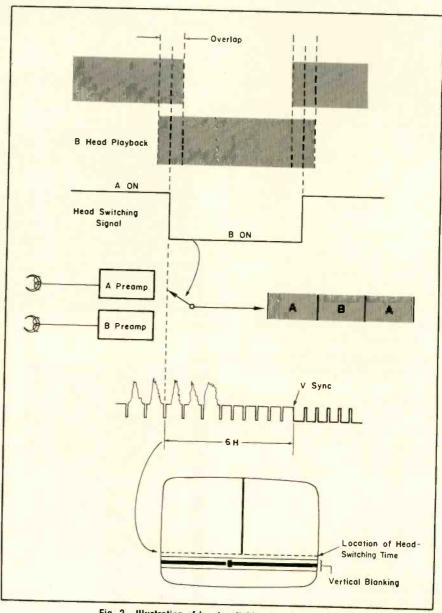
Fig. 2—Illustration of head switching in a two-head helical videotape unit.
