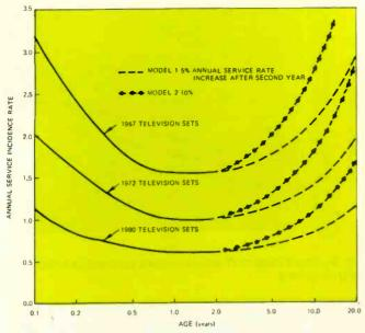
Fig. 4—Models of annual service-incidence rates of 1967, 1972, and 1980 model-year color TV receivers.
