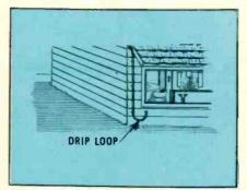
Fig. 9-A drip loop installed where antenna enters house prevents rain from entering house via antenna lead-in.
