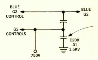
CAUSE: Leaky or shorted C208, in CRT screen grid circuit. About 100K ohms of leakage measured across C208.
