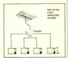
Fig. 12-An example of how an amplified coupler can be used to drive a home MATV system.
