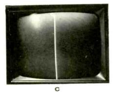
Fig.5—Comparison of horizontal sync recovery times of two color TV receivers. A) Late-model Sony 19-inch receiver. B) Three-year-old Zenith. C) Same Zenith receiver with horizontal AFC filter modified to speed up response time.
