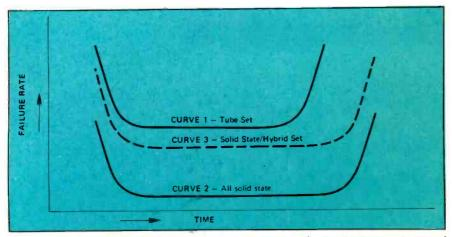
Fig. 3—Typical lifetime failure rates of all-tube, hybrid and early all-solid-state receivers, and later-generation all-solid-state receivers.
