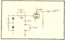
Fig. 7—AFC filter modification illustrated here increased horizontal AFC response time of three-year-old Zenith color receiver from that shown in Fig. 5B to that shown in Fig. 5C.
