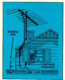
Fig. 6-Lightning protection as provided by lightning arrestor, ground wire and ground rod for twinlead transmission line.
