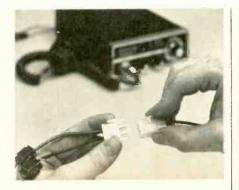
able from Breaker Corp. The new device is designed to prevent equipment theft and make removal for base operations easier. QDC is insulated and polarized with a positive lock between male and female sections and is disengaged by pressure on flexible molded clasps on either side of connector. Sells for \$2.95.
