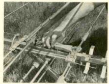
Fig. 7-A matching transformer installed at the antenna when using coaxial cable for transmission line.
