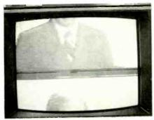
Fig. 3.—Displacement of performer's sleeve just above the vertical blanking bar is indicative of back-tension error in the videotape unit—an error which causes the switch from head B to head A to occur too early.
