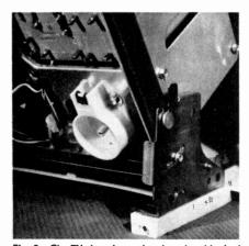
Flg. 2—The TV chassis can be placed and locked in several positions by a "slotted pivot" groove located at the bottom of the chassis.
