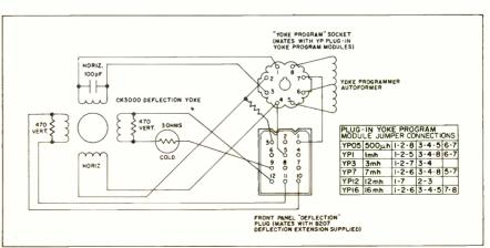
Schematic diagram of deflection circuit employing a Yoke Programmer Autoformer.
