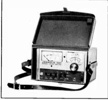
Fig. 1—A typical field-strength meter.
