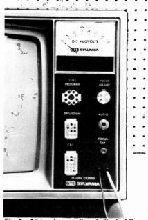
Fig. 5—All input connections to the test jig are located on the front panel and are of the plug-in type.
