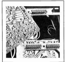
Fig. 3—Module connections are made through a pin and socket arrangement and the master board is eliminated.
