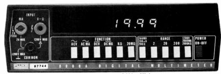
Resolution is 100 microvolts, 100 nanoamps and 100 milliohms
