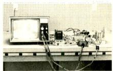
Fig. 3—Photo taken in ETD's test laboratory showing the test jig in operation, producing a well proportioned TV picture.
