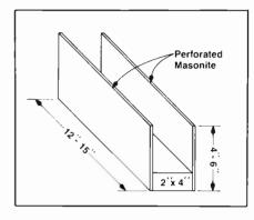
Fig. 6—Auto radio holder devised by Frank Weisel, Norfolk, Virginia.
