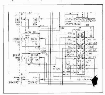
before pulling the control cluster to measure resistor R152. For example, substitute the RGB/Chroma module; also, check the 800 volt B+ supply for the CRT screen elements.
