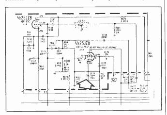
(50 mfd, 150 volts). This capacitor is in the cathode circuit of the vertical output tube. Replace it with Part No. 67A27-8.
