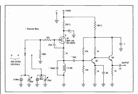
Fig. 3—Crystal-controlled, 1-to-20MHz oscillator.
