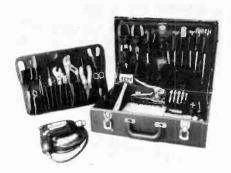
made by leading manufacturers. There are tools for hardwire systems as well as items needed for the adjustment and servicing of ultrasonic, radar, infrared, CCTV, and other advanced detectors. Most of the tools are mounted on two removable pallets. The pallets in turn are mounted in a deluxe attache case.
