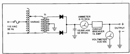
Fig. 1—Power supply for car radio/tape player servicing.
