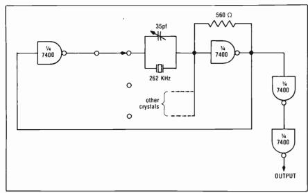
Fig. 4—Crystal-controlled, 100-KHz to 2000-KHz oscillator, most of the circuitry of which is contained in a single type SN7400 TTL integrated circuit. (Crystals for this oscillator circuit and that in Fig. 3 are available from a number of sources, including JAN Crystals, 2400 Crystal Dr., Fort Meyers, Florida 33901. Specify for a 32-pf load and whatever type of holder you want—type HC6/V or HC25 are recommended.)
