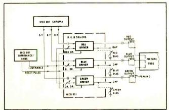
Fig. 5—Diagram of the Red, Green, Blue Driver Module MCD001 and associated systems.
