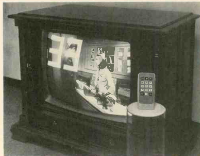
Fig. 6—Magnavox color TV sets equipped with the "STAR" remote-control system display the channel number on the screen in the form of a six-inch-high digit. Shown on right of the photo is the "STAR" remote control unit with a control panel which resembles that of an electronic calculator.
