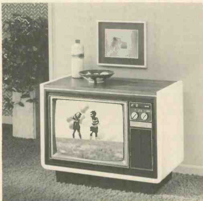
Fig. 13—RCA's Model GT803 color TV receiver employs the CTC68 chassis and an electronic digital channel indicator.
