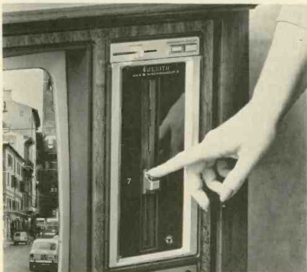
Fig. 19—Zenith's solid-state electronic tuning system and associated VHF/UHF slide-type channel selector.
