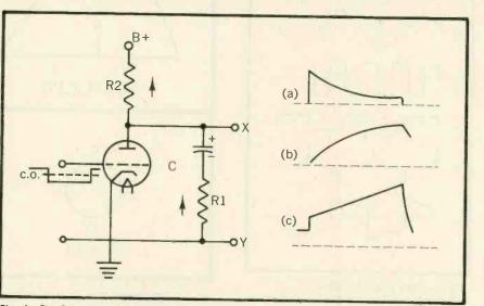
Fig. 4-The formation of a trapezoidal voltage waveform using an active circuit.
