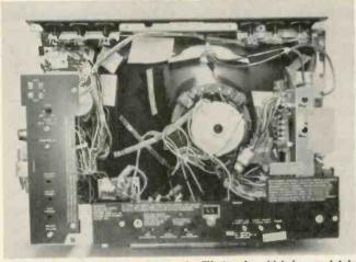
Rear view of the "U" shaped T982 color-TV chassis, which is completely exposed with the cabinet cover removed.
