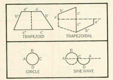
Fig. 2—Components of a trapezoidal waveform can be analyzed in the same manner as those of a sine wave.
