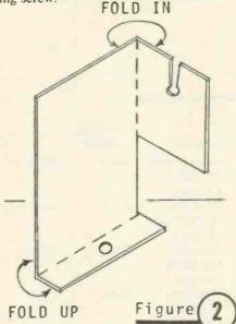
Providing the tripler white focus lead is routed toward the back of set, position the lead through the notch provided in the insulating barrier as shown. Should the focus lead be routed to the front of set, the lead is not positioned through the notch in insulating barrier.
