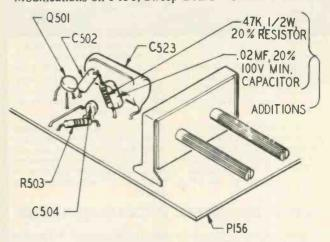
from the board the end of capacitor C502 which is close to the dual control. Insert between the end of capacitor C502 and the hole from which it was removed a 47K,  $\frac{1}{2}$  w 20% resistor and a .02µf 20% 100v minimum capacicontinued on page 44
