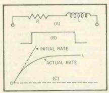
Fig. 5—The resulting current with the application of a trapezoidal voltage waveform to a CRT yoke.
