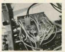
The Videomatic board was redesigned because of the location of the PRESET controls and is not pluggable as was the earlier version.
