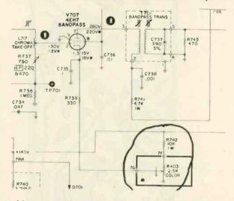
and in one case the COLOR control was damaged. The failure resulted from current flow in excess of the power rating of the resistor.
