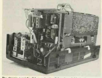
The chassis consists of two main circuit boards and 14 plug-in modules. The Signal board assembly is mounted vertically and the Scan board mounted horizontally.
