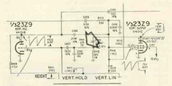
may not show any external evidence of failure. Replace it with the same type and value, Admiral Part No. 60A14-473.
