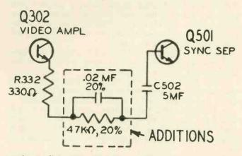
tor in parallel. Change transistor Q501 to an 86X0048-001 transistor. Cut foil on the PW500 board as shown to eliminate a common-ground path between the heater returns and APC circuits.
