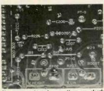
The components and connections are clearly roadmapped with identification numbers to aid any required servicing.
