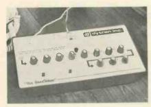
line junction block with the supplied adapter. The unit continues to redial until the call is completed and listener uses the remote shut-off signal. It is powered by four standard "D" cells and measures 16 in. long by 7 in. wide by 3 in. deep. Dytron Inc.
