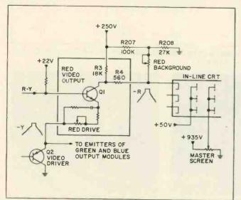
Simplified schematic of the Red Video Output circuit employed in the T982 color-TV chassis. Courtesy of Magnavox.
