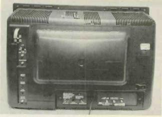
Rear view of the color-TV set showing service adjustments, plus the customer adjustments at the top rear of the cabinet.
