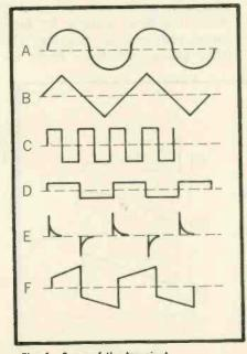
Fig. 1—Some of the transient waveforms found in circuitry currently requiring servicing.
