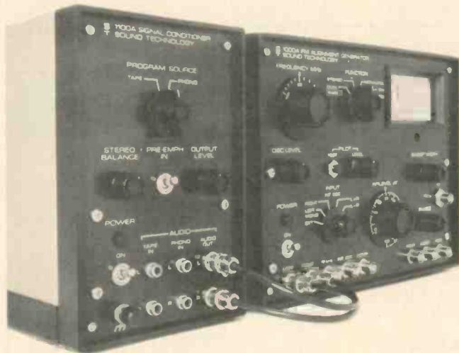
This Sound Technology 1100A/1000A system simulates a high-quality FM broadcast station. It thus lets a dealer demonstrate overall receiver performance using a turntable or tape recorder and whatever program material he or his customer prefers.
