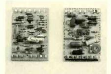
The Horizontal dura-module (9-90) shown at the left, contains all of the transistors in the horizontal circuit except for the output transistor. The Video Processor module (9-87) is shown in right of the picture.
