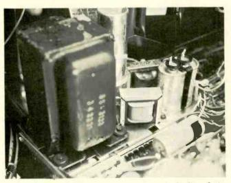
The voltage regulating type transformer employed in the Power-Sentry system appears a little higher and larger than the conventional-type power transformer.
