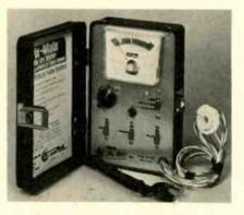
take on every call. The picture tube checker (Telematic Pix Mate) checks each gun for emission, leakage and shorts, with a legible three-color scale and line adjustment for accuracy. It reportedly checks all 90° tubes. An adapter is available for 70° picture tubes. TeleMatic.
