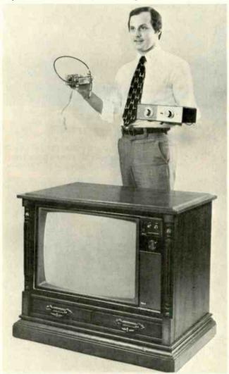
A compact, solid-state electronics unit (left) is now incorporated into the new ready-for-cable TV sets to replace the separate 24-channel selector (right) previously required for cable TV systems. RCA's new line of 25-in. (measured diagonally) color-TV features wireless remote control, AFT, and instant picture—all features previously unavailable with cable reception. Courtesy of RCA Corp. them and 100-percent solid-state RCA XL-100 receivers.
