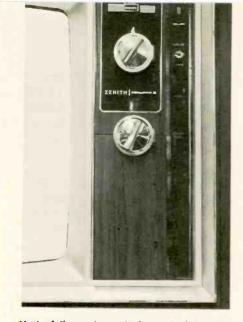
Most of the customer tuning controls are located on the front panel with the exception of the PICTURE PEAKING and  $\blacksquare$ ORIZONTAL HOLD. The AFC, CHROMATIC and ON/OFF are pushbutton type switches.
