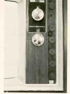
After removing one screw and prying off the control panel cover, an insulated screwdriver is inserted through the center holes of the customer controls to adjust the factory preset controls.
