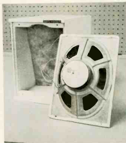
The speaker and baffle appear to be made of a single piece of cast white metal. Note the single sheet of sound-absorbing material that is pressed into position between the speaker area and the electronic circuitry.
