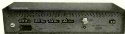
Rear view of Quadraline receiver showing its four-channel speaker output terminals, four-channel tape output terminals, four-channel tape input terminals, four-channel phonograph input terminals, four-channel FM decoder terminal, 300Ω FM antenna terminal, rear-channel BALANCE control and accessory power outlet.
