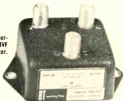
Fig. 11—Using MUVF multiplexer as VHF attenuator results in 40dB of attenuation of undesired strong VHF signal before application to UHF/VHF converter.
