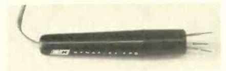
The FP-3 test probe for making in-circuit measurements with the curve tracer.
