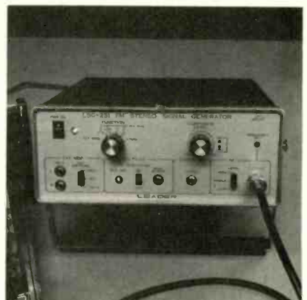
Close-up view of Leader's Model LSG-231 FM Stereo Signal Generator. Note the FUNCTION switch which can be rotated for EXT. MOD, L - R, L + R, L, R, and 67kHz.
