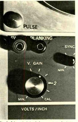
Fig. 3—Pulse output terminals on a scope showing the "sweep" and "blanking" pulse binding posts.
