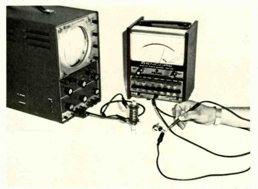
Fig. 14—An electronic technician is shown measuring the resistance of a potentiometer to determime the ac resistance of the coil.
