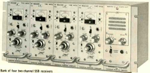
for use on ships or at shore stations. Courtesy of Kaar Electronics Corp.
