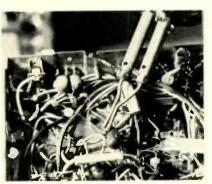
Fig. 3—Heating a suspect component with the tip of your soldering iron may indicate if it is defective.
