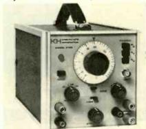
1000:1 tuning range of the dial. Output is said to be controlled by a twoposition dB step attenuator and amplitude vernier, providing both a  $50\Omega$ single ended and a  $600\Omega$  balanced output. The outputs reportedly provide 15v p-p and 30v p-p respectively, plus a 1v auxiliary output. Krohn-Hite Corp.
