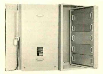
Marine radiotelephone system for larger vessels. Rack contains both VHF/FM and MF-HF/SSB transmitters and receivers. Courtesy of COMCO, a subsidiary of E. F. Johnson Co.
