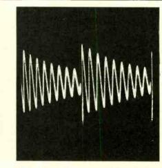
Fig. 8—Wave train of a good horizontal-output transformer using a pencil-type signal injector as a pulse source.
