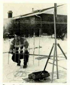
The collapsible mast in the foreground fits handily in the service truck, ready for use wherever Joe Barno goes. The 5-ft. sections of mast permit quick, convenient height adjustments of the test antenna.
