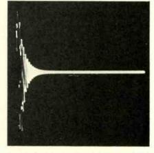
Fig. 9—A defective horizontal-output transformer. Note the very short wave train.
