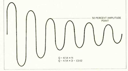
Fig. 13—The wave train may be used to determine the Q of a coil. In the equation, N equals the number of cycles up to the 50 percent point.
