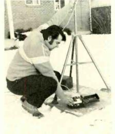
While rotating the mast and antenna with his left hand, Joe Barno watches the field strength meter to find the direction from which maximum signal strength is received.
