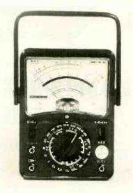
HM-310, VOM/Transistor Tester is a self-contained three-in-one VOM/ Transistor/Capacitance Tester featuring 100K per volt, taut-band movement, 3-in. mirrored scale and burn-out protection. Measurement capabilities include: AC and dc volts, resistance, ac and dc current, dB, and capacitance transistor alpha, beta and leakage current. The unit measures  $2\frac{1}{2}$  by  $5\frac{1}{16}$  by  $6\frac{1}{2}$  in. and weighs 2 lb. hme Electronics Inc.
