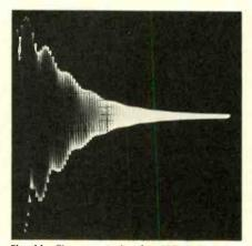
Fig. 11—The wave train of a 455kHz IF transformer.
