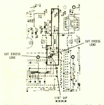
It is strongly recommended that should any of the subject chassis come in for shop service regardless of reason, check the two points in order to prevent any possible future failure.
