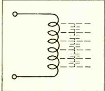
Fig. 2—A coil represented schematically to show capacitance between layers of wire.
