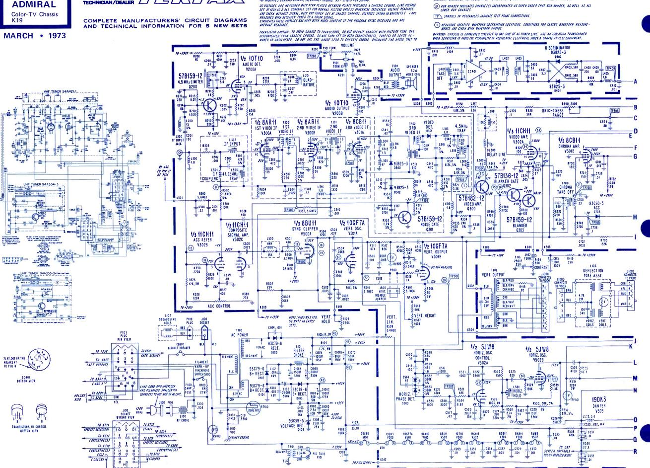
NOTES: UNLESS OTHERWISE SPECIFIED: RESISTANCE VALUES ARE IN OHNS, ION, 1/2 MATT; CAPACITANCE VALUES 1 OR HIGHER ARE IN PF; CAPACITANCE VALUES LESS THAN 1 ARE IN UF; INDUCTANCE VALUES ARE IN UM. #INDUCATES CHASSIS GROUND, FT CABINET GROUND, H2 + CYCLES PER SECOND.
