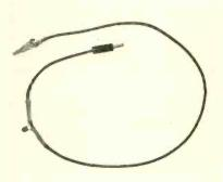
Fig. 4—Ringing lead made up by putting a 15pf capacitor in series with a wire and terminating it with an alligator clip.
