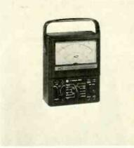
0-250v ac in four ranges. Ohms:  $R \times 1$ ,  $R \times 100$ ,  $R \times 10,000$ . All ranges except the 10a and 1000v dc ranges are protected by the electronic overload system and the relay contacts are protected by a 3a fuse in the input circuit. The unit measures 51/4 by 7 by 31/8 in. deep and weighs 3 lb. Dynascan Corp.
