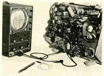
Fig. 1—Ringing test of a horizontal-output transformer using a penciltype signal injector.
