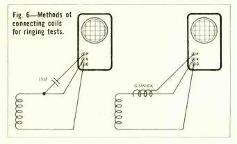
train on the scope.) The vertical input of the scope is also connected to this cap, while the ground clip of the scope is attached to the chassis, or B- in ac/dc sets. This arrangement of components (as first shown in Fig. 1) produces very satisfactory ringing patterns (Fig. 8).
