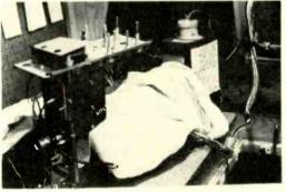
Fig. 2.—For the intermittent that occurs after warm up, it is best to place a flameproof blanket over the chassis.
