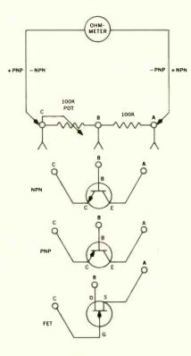
transistor or FET can be accurately tested. And with some experience, gain can be approximated, transistors can be matched, etc.
