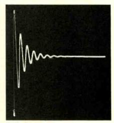
Fig 12—The wave train of a choke.
