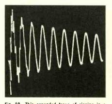
Fig. 10—This expanded trace of ringing in a horizontal-output transformer shows oscillations riding on top of the wave train.
