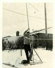
Up goes the top section as Joe Barno prepares to test signal strength with an antenna cut to Channel 9. The home owner at this location has had a weak signal problem on this channel.
