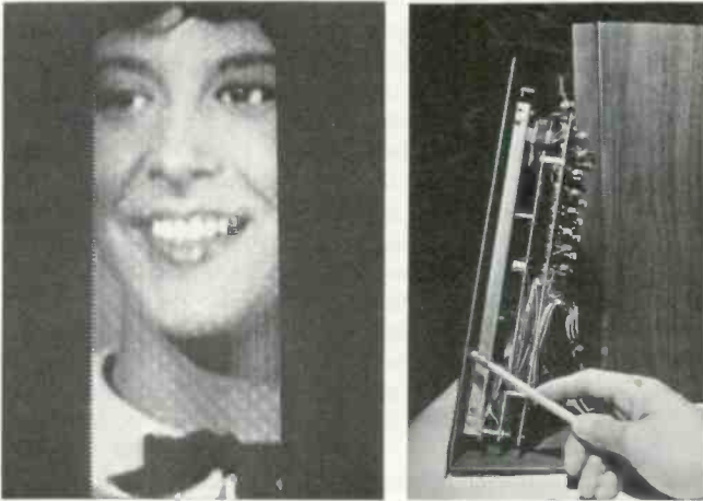
Front and side views of the thin-panel gas-discharge display. Without the associated electronics, the panel is \frac{5}{8} -in. thick.
