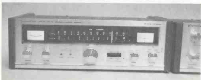
Fig. 2—FM Multipath signals for the scope were obtained from Kenwood's Model KT-7001 AM-FM Stereo Tuner.
