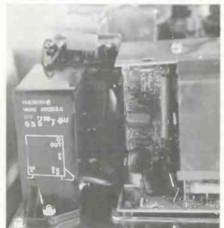
A hermetically sealed solid-state quadrupler reduces the required pulse from about 23kv to 6kv.
