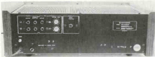
Fig. 5—Input and output terminals at the back of the scope.
