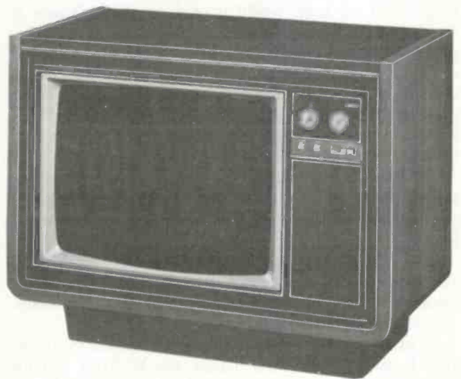
RCA's Royalton, Model GR-802, color-TV set employs a tempered black architectural glass top. Courtesy of RCA Sales Corp.
