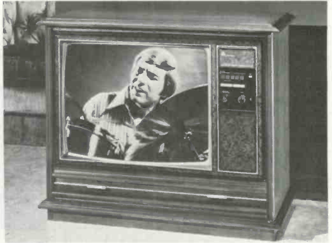
Motorola's Model WU9106JW color-TV set, featuring an all solid-state chassis with plug-in modules. Courtesy of Motorola.
