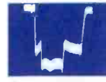
4 1.8V P/P, 15,750Hz Hor. Sync. Pulse Showing 4.5MHz Trap out of Adj.
