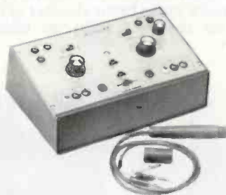
LTC-905 CURVE TRACER Test transistors, triacs, SCR's, diodes, FET's, & MOSFET's, in or out of circuit, 8 precise volt or amp. steps. Has horiz. length adj. to 100V sweep. With special probe. $119.95
