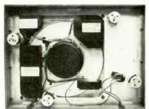
Fig. 6-The inside of the turntable base assembly.
