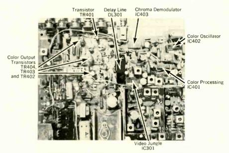
The luminance and chrominance circuits consisting of three IC's and four transistors are located on one panel.
