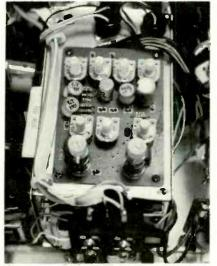
The dynamic convergence panel is located above the chassis, simplifying color adjust-
