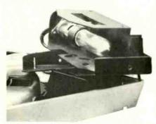
Fig. 21-The optical system has been opened to permit removing the neon lamp.
