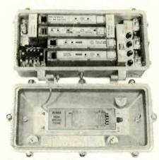
Fig. 2-Trunk amplifier station.
