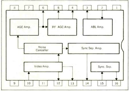
Block diagram of the "video jungle," IC301, containing the noise canceller, sync separator, AGC, and video amplifier circuitry. Courtesy of Panasonic.
