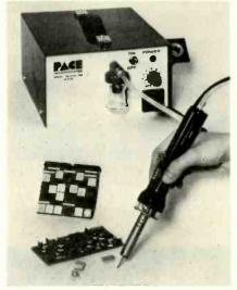
supply. Controls on the front panel of the power source permit controlling the temperature to any desired level up to 1000°F. Solder joints are melted with a coaxial tubular tip. Then, the foot pedal, connected directly to the power source, can be depressed to provide an instantaneous continuous vacuum. The continuous vacuum removes the molten solder and then cools the solder joint area to prevent the resweating of component leads to hole and pad areas. Price: \$249.00. Pace Inc.
