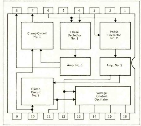
Block diagram of the circuits employed in the color oscillator integrated circuit, IC402. Courtesy of Panasonic.
