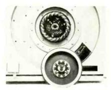
Fig. 13-Top of disassembled dc turntable motor.
