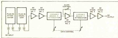
Fig. 3-Essentials of trunk amplifier module.
