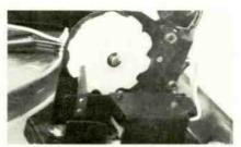
Fig. 9-Side view of the mechanical systems required for the POWER and SPEED-CONTROL switches.
