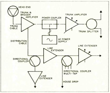
Fig. 1—A typical CATV system.
