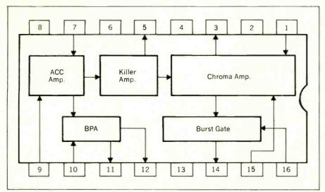
Block diagram of the circuits employed in the color processing integrated circuit, IC401. Courtesy of Panasonic.
