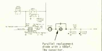
diode. To prevent such failures, make certain a 680pf, 1kv capacitor, Stock No. 113165, is connected in parallel with the diode replacement.
