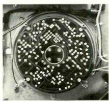
Fig. 11-Bottom of circuit board used for sequencing the stator electromagnets.
