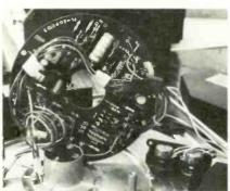
Fig. 12-Top of circuit board used for sequencing the stator electromagnets.
