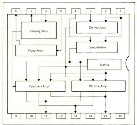
Block diagram of the circuits employed in the chroma demodulator integrated circuit IC403. Courtesy of Panasonic.
