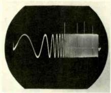
on the equalizer circuits, and the job is done. The audio range of the unit is from 60Hz to 15KHz with marker pulses at 1, 3, 5, 10 and 15KHz. Pacific Transducer Corp.
