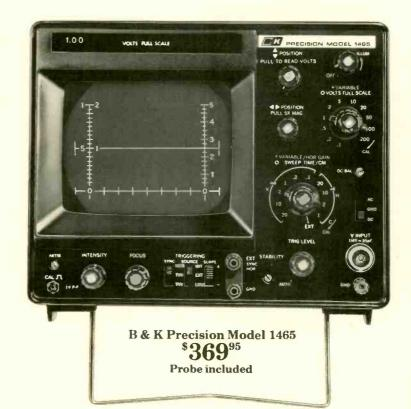
overlay is illuminated on either side of the scope screen. The scale corresponds to the full scale voltage indicator in the bezel.
