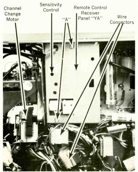
To replace the YA panel, remove two 1/4-in, hex head screws (A) and disconnect the microphone cable. Disconnect two plug-in cables, a 10-prong and 12-prong connector, and then slip the panel
