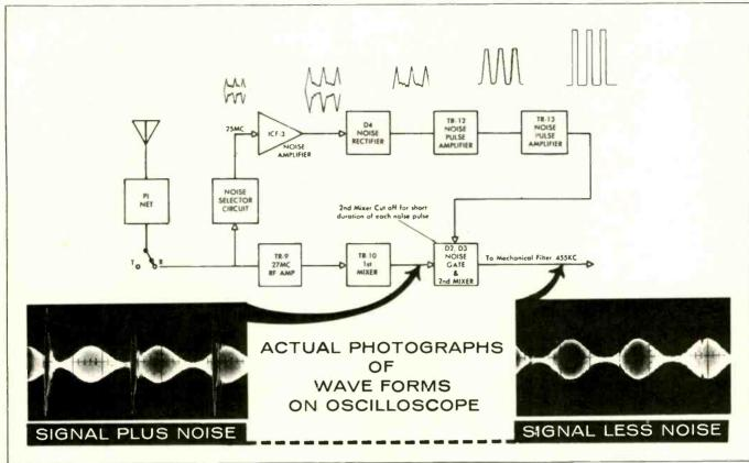
Fig. 5-RF Noise silencer circuit and waveforms. Courtesy of Lafayette Radio Electronics Corp.
