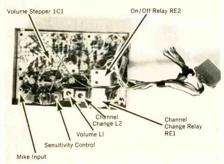
Most of the remote control receiver circuitry is located on a separate YA plug-in panel.
