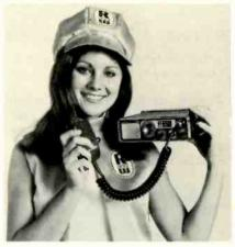
preset to the more commonly used frequencies, but can be reset in the field following the instructions provided with the transceiver. A front panel power selector switch allows a choice of power output of 0.1w, 1.0w or 10w. The power requirement is  $13.5v \ dc \pm 10\%$  at 2.42a. The unit has  $12 \ channel \ capability \ with a selector switch control. Ross and White Co.$
