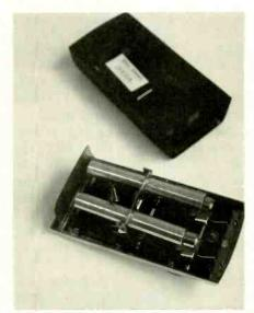
Inside view of the transmitter showing the mechanically resonant rods, which act as a transducer to convert mechanical energy to acoustical energy.
