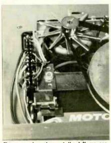
The many wires shown at the left are connected to the cartridge MODE switch. Because of the slot in the four-channel cartridge, inserting the cartridge does not cause the lever to press against the switch—leaving it in the four-channel mode.
