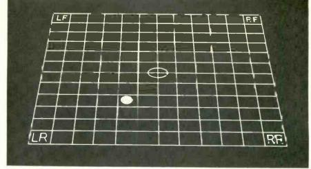
Four-channel BALANCE control grid system as seen through the front panel. The grid pattern (illuminated in green) represents the room in which the tape player is used, the corners of the grid representing speaker locations. The position of the dot (illuminated in red) can be moved across the grid to a location corresponding to your position within the room—the location for which you want the speakers balanced.
