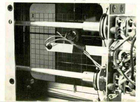
Upon peering through the panel opening through which the tape cartridge is inserted, we can see the TRACK switch, tape guide, tape head, cartridge eject arm, tape drive capstan and POWER switch.
