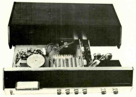
After removing six bolts from the underside of the cabinet, the chassis can be slid out the front of the cabinet.
