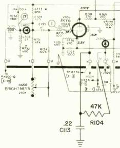
the 260ma current cannot be obtained, either change resistor R731 to 27K or bridge it with a 68K resistor.
