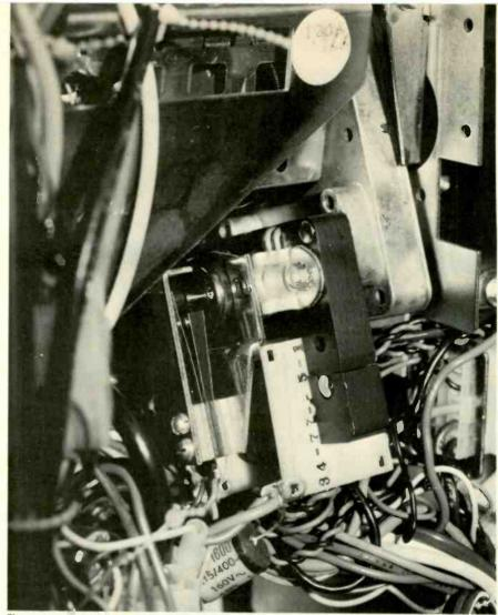
The mute switch is located at the rear of the channel-change motor armature. This switch blanks the picture and mutes the audio signal during tuner rotation.
