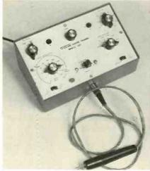
circuit board. This instrument checks both bi-polar and field effect transistors and is designed to operate in conjunction with any general purpose scope to display a six-line family of curves. It has two sockets for testing and matching transistors out-of-circuit and two types of probes for in-circuit testing. Price is \$150.00 including both probes. Testline Instruments.
