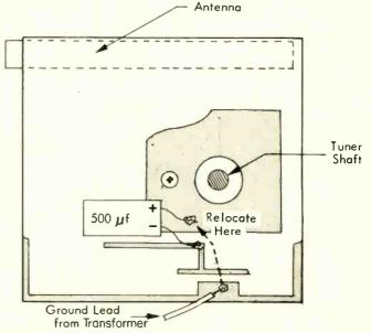
down transformer and reconnect it to the same solder connection used for the grounded-positive lead from the 500 µf filter capacitor, as shown in the illustration.
