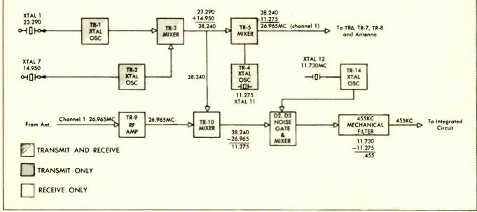
Fig. 3—Frequency conversion for Channel One. Courtesy of Latayette Radio Electronics Corp.
