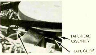
ARM FOR SUPPORTING TAPE-HEAD ASSEMBLY AS IT MOVES UP AND DOWN
