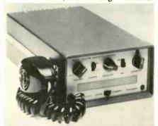
changing. It employs a broadband FET front-end design which provides an average sensitivity of  $0.35\mu v$  over the entire marine band. Airmarc Corp.
