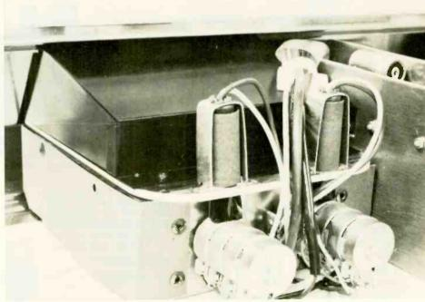
Two lamps mounted at the back of the frame housing the grid pattern are used to illuminate it. A filter around each bulb causes the pattern to appear green.
