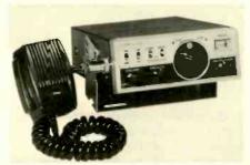
that enables the user to monitor the emergency channel and any other selected channel simultaneously. The unit continuously scans both channels but locks in on the first signal. It is all solid-state and features a noise blanker
