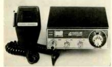
in, power leads are quick disconnect and jacks are conveniently placed for PA and remote speaker. The Puma 23 receiver is reportedly rated at 0.5 µv sensitivity and has a crystal filter and high performance automatic noise limiter. Price: \$114.95. Pearce-Simpson Div., Gladding Corp.
