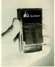
The remote control transmitter is a compact unit, with two push buttons-one turns the TV set ON or OFF and changes the volume level, while the other changes channels.
