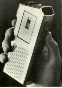
Powered by a standard 9v battery, the unit weighs less than 20 oz. Its features include visual indexing, automatic sound LEVEL control and separate built-in microphone and speaker elements. Philips Business Systems Inc.
