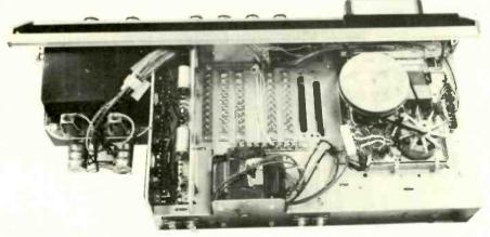
Top view of tape-player chassis with tape cartridge in place.
