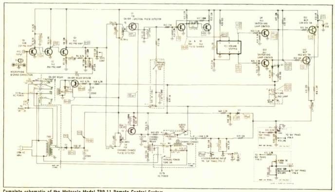
Complete schematic of the Motorola Model TRR-11 Remote Control System.
