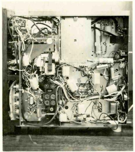
Side view of Motorola's color-TV chassis TS938 with the remote receiver removed.
