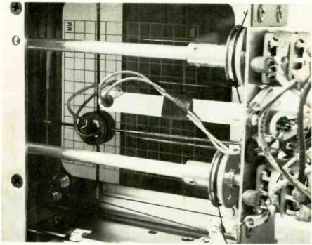
Dial cords attached to the FRONT-TO-REAR BALANCE control and LEFT-TO-RIGHT BALANCE control are used to vary the position of a lamp housed beneath the transparent grid pattern. A red filter on the underside of the grid pattern causes the lamp to appear as a red dot.
