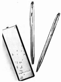
incoming call. The unit automatically resets itself to the "listen" mode after each page is received, so once it is turned ON, it reportedly needs no handling. A special built-in "memory" option is designed to permit the user to delay receipt of a page when its interruption might be inopportune. Motorola, Inc.
