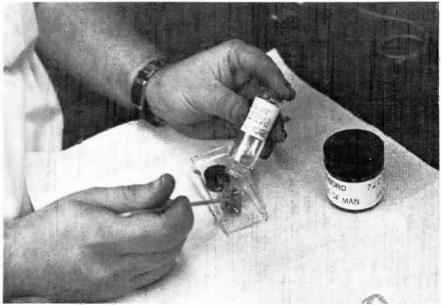
Fig. 1-Combining the two-part conductive epoxy in a two-to-one ratio.
