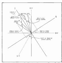
Fig. 4—Vectors indicate the results of the chroma phase shifts in Admiral's color monitor circuit. Courtesy of Admiral Corp.
