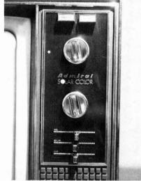
Fig. 2—Front control panel showing the new AUTOMATIC FINE TUNING/COLOR MONITOR control (top right). The VOLUME, TINT and COLOR controls are the slide throttle type.
