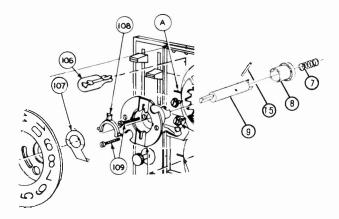
• Spring No. 107 was changed from 19A384-1 to a heavier spring No. 19A384-2 (or two 19A384-1). See illustration.
