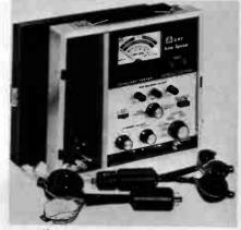
as well. All functions, including filament voltage setting, gun balance setting, shorts test, shorts removal, emission check, and three rejuvenation positions are reportedly covered with a single switch. The unit is housed in a brushed steel and vinylclad carrying case, with setup book included. Price: \$140.00. Sencore, Inc.
