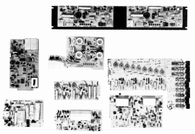
Circuit boards used in Heath's AR-1500 receiver. Top: Left and right channel output amplifier circuit boards mounted on heat sink. Middle right: Input preamplifier circuit board. Bottom right: FM-IF circuit board. Bottom center: AM-IF circuit board. Bottom left: Power supply circuit board. Top left: Multiplex circuit board. Top center: Control circuit board. Lower center: Phonograph preamplifier circuit board.
