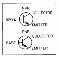
Basic transistor schematic symbols.
