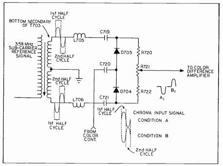
Fig. 5—The color demodulator circuits consist of phase sensitive detectors employing two diodes. Courtesy of Admiral Corp.
