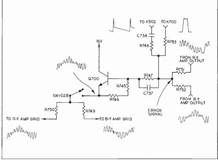
Fig. 3—Schematic of the matrix-type color monitor circuit, which produces a correction signal fed back to the demodulator's output to restore proper color phase. Courtesy of Admiral Corp.
