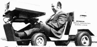
The vehicle measures signal strength and noise levels of several antenna models which are buried in a test roadway. Based on test results, GTE Sylvania's Sociosystems Products Organization will recommend antenna models and related equipment, as well as techniques, for the development of a highway communications system whereby drivers and authorities can exchange messages.
