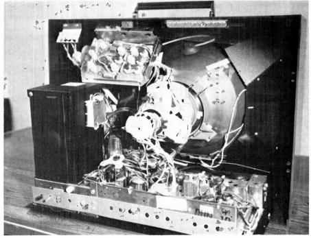
Rear view of the Admiral 1K18-1A color-TV chassis, which is exposed after removing the cabinet back.
