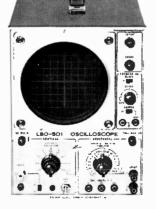
Now the wave shape is locked in and continuously displayed. Now you can look at a waveform containing high and low frequency components. Now you can determine voltage directly and instantly.
