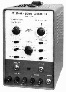
justable frequency range of 75 to 110MHz. Rated separation is over 30dB from 50Hz to 15kHz. The instrument checks separation and balance in FM receivers and tuners and also serves as a sweep-marker for 10.7MHz FM and IF alignments. It features a 115-230v, 50/60Hz dual power supply, measures  $10\frac{1}{2}$  in. H by 7 in. W by 11 in. D and weighs  $13\frac{1}{2}$ lb. Accessories include a  $300\Omega$ , 75 $\Omega$ (open) cable. Price: \$175.00. Leader Instruments Corp.
