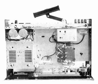
Top view of receiver chassis with circuit boards removed.
