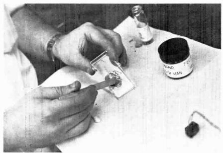
Fig. 2—Manufacturer's specifications require that both parts be completely mixed with a wooden stirrer.
