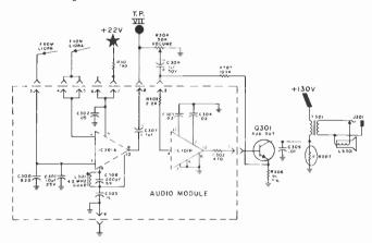
The IC contains a detector section and an audio amplifier section. The detector circuit operates much the same as the quadrature detector used in tube-type receivers. The quad coil, L301, is the only tuning adjustment on the module, and it should be tuned for maximum audio.
