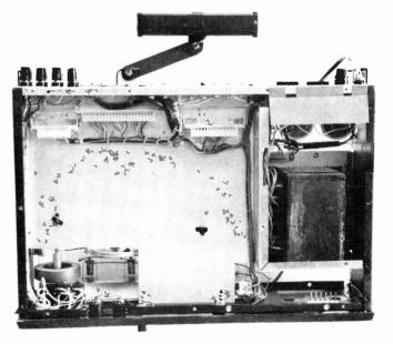
Bottom view of receiver chassis with circuit boards removed.
