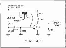
Fig. 1—A simplified schematic of the solidstate noise gate circuit employing one transistor and one diode. Courtesy of Admiral Corp.
