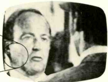
By substituting the transistorized antenna for the rabbit ears (and operating its elements at the same length as the rabbit ears), a much better picture is received from the same station.
