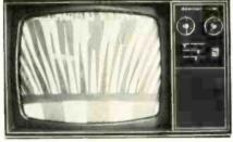
Fig. 17—TV picture produced when analyst vertical-grid-drive signal is fed to grid of vertical "oscillator tube."
