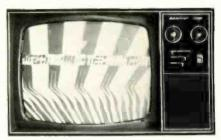
Fig. 18-TV picture produced when analyst sync signal is fed to cathode of vertical "oscillator tube."
