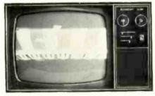
Fig. 16—TV picture produced when analyst sync signal is fed to grid of vertical "oscillator tube."
