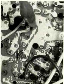
Fig. 3-Injecting analyst sync signal to grid of horizontal-oscillator-control tube.
