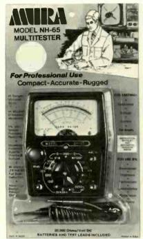
D'Arsonval movement, diode overload protection to prevent burnout and 50µa 0.25vdc full scale deflection. The VOM reportedly contains an advanced design printed circuit and 1 percent wire-wound resistors throughout. Price \$15.95 user net including batteries, test leads and operating instructions. Mura.
