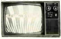
Fig. 20-TV picture produced when analyst vertical-grid-drive signal is fed to grid of vertical "output tube."
