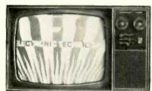
Fig. 5-TV picture produced when analyst sync signal is fed to grid of horizontal-oscillator tube
