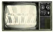
Fig. 24—TV picture produced when vertical scan signal is produced solely by applying analyst vertical-grid-drive signal to grid of vertical "output tube."
