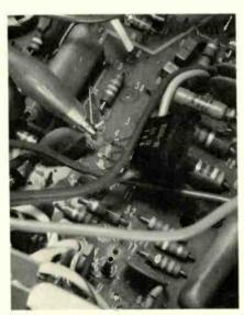
Fig. 1—Capacitor leading to horizontal phase detector is disconnected from TV set's sync amplifier and fed sync signal from analyst.
