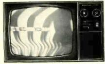
Fig. 2—TV picture produced when analyst sync signal is fed through capacitor to horizontal phase detector.
