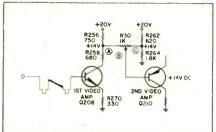
Fig. 3-The bridge contrast control circuit, employing a dc video amplifier chain.
