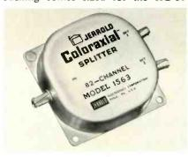
cable. An expansion tool, ET-659, is supplied to expand the cable bushing for CAC or CAC-6 cable size. The 1563 splitter is said to have a splitting loss rated at 3.5dB for VHF and 3.8dB for UHF, with 18dB isolation between outputs and a frequency range of 54 to 890MHz. List price per unit is \$6.95. Jerrold.
