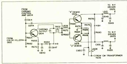
Fig. 7—The X and Z color demodulator circuits.
