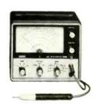
EICO 240 Solid-State FET-TVM. \$59.95 kit, \$79.95 wired. AC or battery operated. 7 ranges each + and - DC volts, peak-to-peak AC volts, ohms. 10 turn zero adjust pot. 4-1/2" 200 μA meter. response to 2 MHz (to 250 MHz with optional r-f probe).
