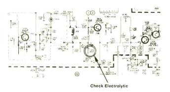
20 µf 15v electrolytic, RCA stock No. 121995) changing value. Possible symptoms include: video "smear"; video "bends"; unstable sync; or various combinations of these symptoms. In addition, the symptom may vary with the brightness control setting.
