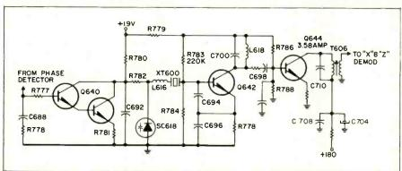
Fig. 4—The 3.58MHz CW oscillator utilizes a modified Clapp configuration.
