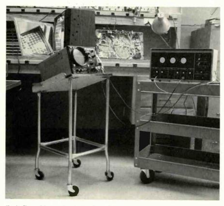
Fig. 1—The usefulness of B & K's Model 1077B Television Analyst is demonstrated with the aid of B & K's Precision Model 1460 Triggered-Sweep Scope and an Admiral T7K10-1C Chassis portable Color-TV set. For added convenience, the scope is used on an Easy-Up Scope Cart.
