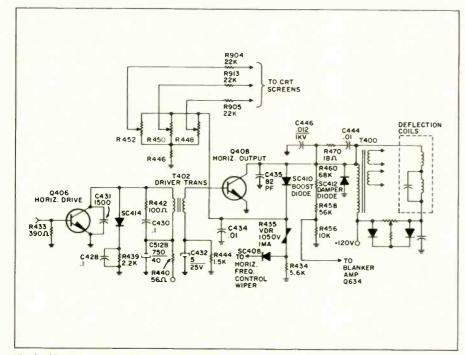
Fig. 8—The solid-state horizontal driver and output circuit.
