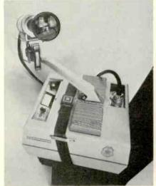
This system, consisting of a zoom-lens camera and solid-state transmitter, can provide law enforcement and public safety officials with live CCTV surveillance from a helicopter.
