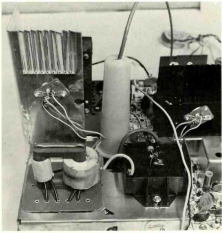
Fig. 1-The horizontal output transformer and high-voltage tripler circuit employed on Sylvania's E01 Color-TV Chassis.
