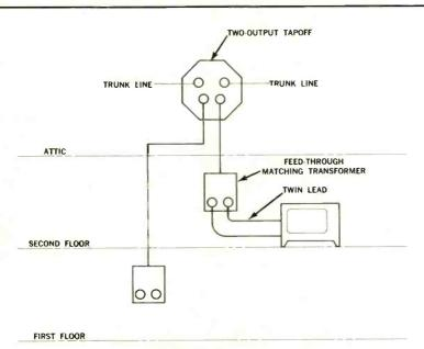
Fig. 3—The distribution system for this typical two-story, 80-room motel or school.
