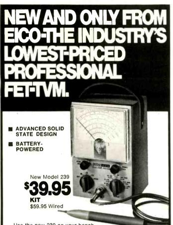
Use the new 239 on your bench or in the field. Checks semiconductor and vacuum tube circuits. 11 Megohm DC input impedance. Reads AC rms and DC voltages in seven 10db steps from 1 to 1000 volts on large 41/2" meter. Measures and reads peak-to-peak AC to 2800 volts. Check resistance from  $0.2\Omega$  to 1000 M $\Omega$  on seven ranges. Includes exclusive tlme-saving Uniprobe.
