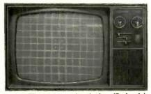
Fig. 8-TV picture produced when IF signal is fed to collector of second IF transistor.
