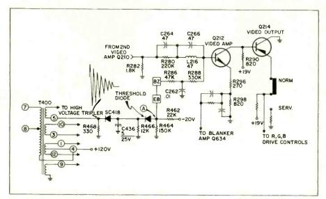
Fig. 2—The brightness limiter is a closed-loop regulator circuit which protects the CRT by limiting the beam current and restricting its emission level.
