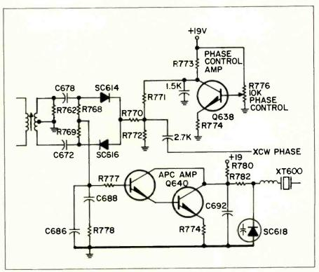
Fig. 5—The 3.58MHz reference oscillator phase control circuit.
