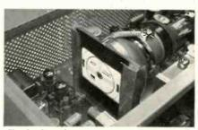
Fig. 2-One of many transparent test patterns that can be used to produce a video signal.
