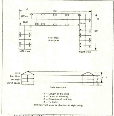
Fig. 2—A typical layout for a motel or school requiring a distribution system.
