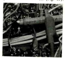
Fig. 12-The input to delay line DLH43 is disconnected and the analyst's video signal applied to its output.
