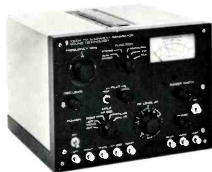
Fig. 3—Sound Technology's 1000A FM Alignment Generator.
