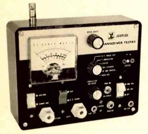
directly in percentage, and standing wave ratios (SWR). Specifications indicate that an audio jack permits headphone monitoring of the transmitted signal, while the tester can also be
