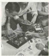
Five technicians work together under the direction of Jim Smith to align a tuner and IF strip.
