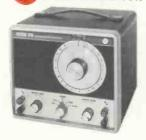
Provides simultaneous sine and square wave outputs. Covers 20 Hz-2MHz, 5 bands. Max. distortion 0.25% Rise time at 20 KHz < 0.1
