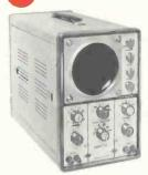
DC-8MHz (usable to 10 MHz). 5" flat-face CRT. Sensitivity 12 MV RMS/CM. Negligible relative H & V phase shift. Excellent curve tracer with Eico 443 (below). Eico 465. Wired \$249.95.
