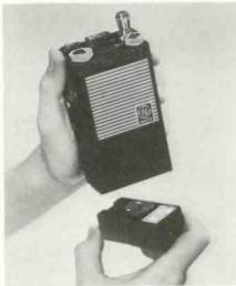
twist-off connector. The Automatic Power Level is a standard feature of all 150MHz models, and it compensates for drop-offs in output power that otherwise would occur if battery voltage decreases with use. The radio circuits are all solid-state, using silicon transistors, thick film hybrid integrated circuitry and modular construction. General Electric.
