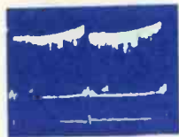
1. PIN 9, V-207 4.5V P-P 2. PIN 8, V-207 4.0V P-P 3. PIN 2, V-207 2.0V P-P
