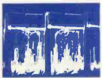
4. PIN 6, V-207 100V P-P 5. PIN 2, V-208 60V P-P 6. PIN 9, V-208 40V P-P
