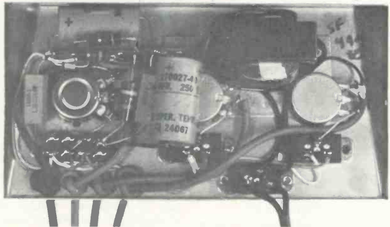
Components inside the dc. bias supply.
