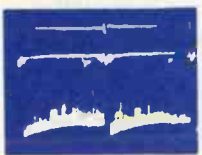
4. PIN 6, V-207 100V P-P 5. PIN 2, V-208 60V P-P 6. PIN 9, V-208 40V P-P
