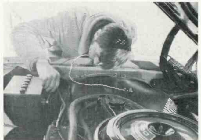
Fig. 3—Bolting fused power line to positive terminal of battery.
