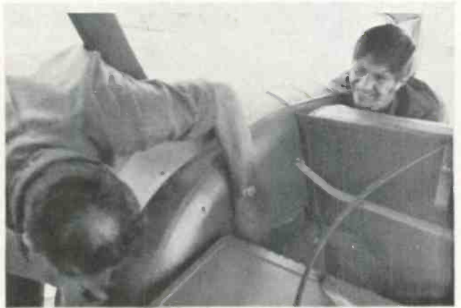
Fig. 13—Running antenna coaxial cable from front to rear.
