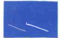
14 V502-6 (Term. L) 1200V P-P Vert. Rate Vertical Output
