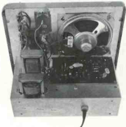
Top inside view of signal tracer.
