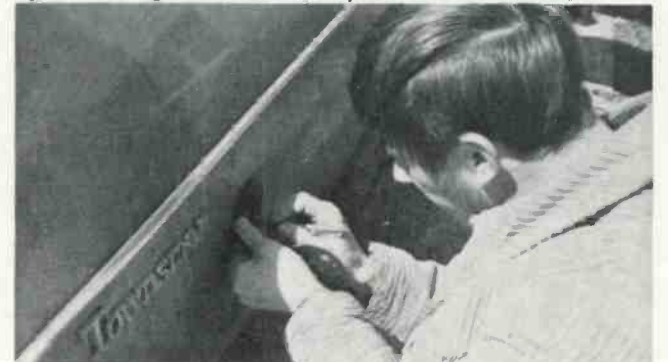
Fig. 11—Marking location of holes required for antenna mount.
