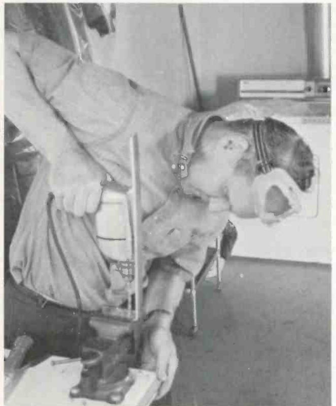
Fig. 8—Drilling mounting holes in legs of side-support brackets.
