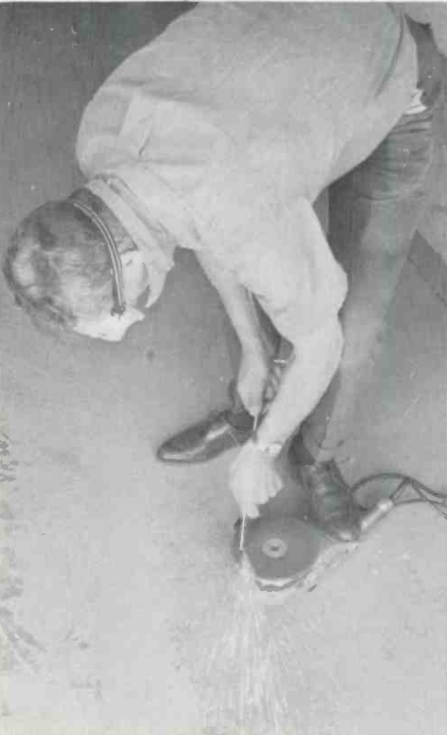
Fig. 7—Sanding a rounded edge at the top of each side-support bracket.
