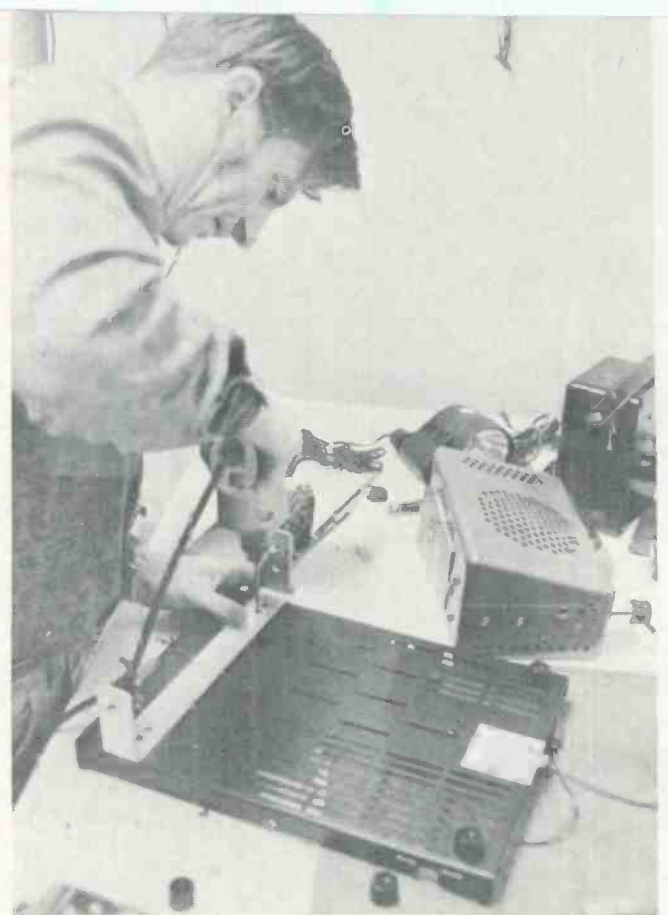
Fig. 9—Drilling holes for mounting additional support brackets to base of transceiver.
