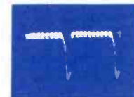
22 V706-2 18V P-P Horiz. Rate Grid Video Output
