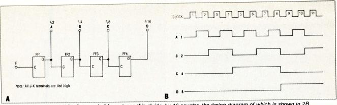
Fig. 2 Cascading four J-K flip flops as in 2A produces this divide by 16 counter, the timing diagram of which is shown in 2B.
