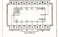
Fig. 9 Pinouts for the TTL series 74160-74163.
