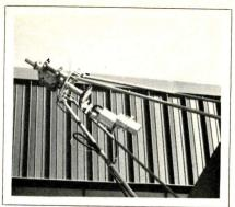
Fig. 7 The rotatable feed horn assembly of the Paraframe R & D antenna.
