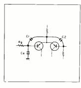
Induced in audio signal routes of the amplifier, such as preamp stage and control circuits. If it is in a differential amplifier, add a capacitor or replace C1 and C2 to achieve a capacitance of C1=C2=47 to 100pF. Also replace Rg and Ca with larger value components, but do not exceed 2.2Kohms and 100pF respectively.
