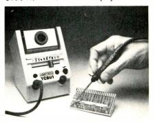
The Antex Soldering Station's 35 watt iron provides temperatures from 350 to 800° F with temperature control reportedly to ±2%. Heat up time is stated to be less than 30 seconds. The soldering iron is positively grounded and weighs less than one ounce. It accepts more than 40 slide on tips from 0.012 to 3/16 inch diameter. The price is \$115.
