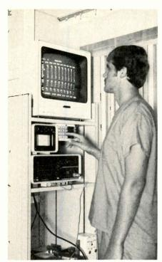
Fig. 2 A scrubbed and suited BMET checks a computer assisted monitor display prior to its application to a patient. (Photo courtesy Roche-Medical Electronics)
