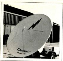
Fig. 6 Dalsat uses an Andrews dish with the feed horn and wave guide rotatable from its base.
