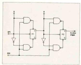
Fig. 5 Two stages of a preset counter using "jam" input.
