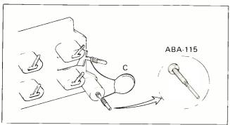
Induced into the grounding wire of turntable output cord. Add a new grounding point near the GND terminal using ABA-115 screw and connect the terminal to the ABA-115 with a thick lead or braided wire.
