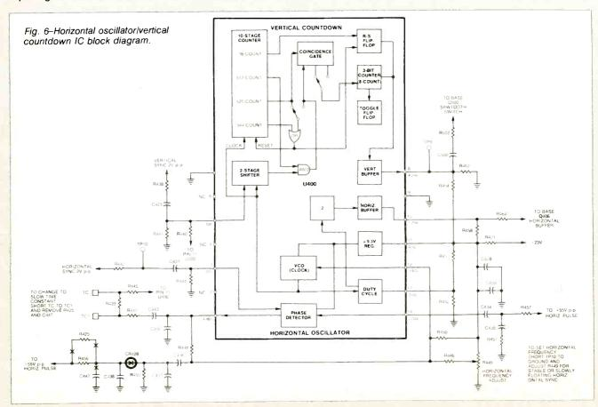
The two modes of operation allow the system to be compatible with nonstandard sync signals. The IC internally switches between the two modes of operation depending upon the type of signal being received. Mode switching occurs after eight consecutive cycles of receiving vertical sync that is either in coincidence or not in coindence with the 525 count from the countdown system.
