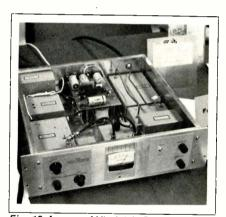
Fig. 10 Avcom of Virginia's PSR-3 satellite video receiver.
