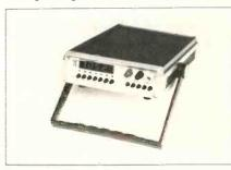
basic accuracy of  $\pm 0.02\%$  of reading  $\pm$  1 digit. Other features include six ranges on each volt/ohms/milliamperes, true RMS ac voltage and current readings, automatic decimal point and polarity indication and the DMM4030 is stated to have high overload protection.
