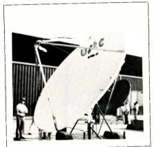
Fig. 3 Paraframe R & D's laminated framework dish with rotatable feed horn for polarization change.
