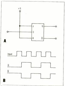
Fig. 1 The J-K flip flop is the basic element in most counters. Figure 1B is the timing diagram for the circuit illustrated in 1A.
