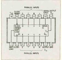
Fig. 9 The 74165 SISO/SIPO device triggers on positive going transitions.
