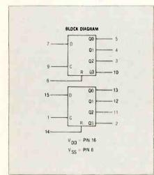
Fig. 11 A dual, four stage SISO/SIPO device, the 4015.
