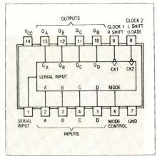
Fig. 6 A basic, four bit PIPO register.
