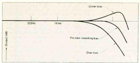
Fig. 8 Graphic representation of how changes in bias level affect the frequency response
