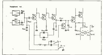
Fig. 3 Pioneer's peak meter circuit
