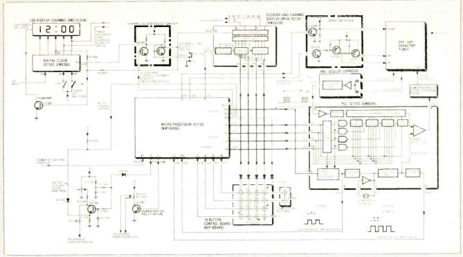
Fig. 2 Synthesizer tuning system block diagram
