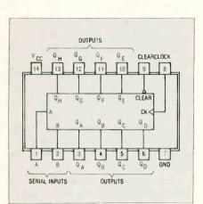
Fig. 8 The eight bit 74164 is usable either as a SIPO or SISO device.
