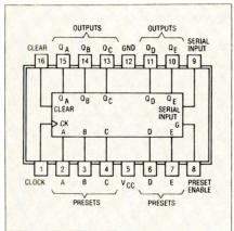
Fig. 7 This 7496 is a "right shifting" PIPO device.
