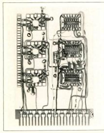
adhesive to a ground plane and in turn have component leads soldered to them. A variety of solder mounts and ground planes are available as are enclosures for prototyping or constructing finished instruments. Components of the system are sold as separate items or in kits.
