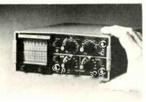
veloped for the Series 1020 to maintain a bright sharp trace; the screen area is  $8 \times 10$ , 5mm divisions. Input sensitivity ranges from 0.005v/division to 2v/ division and sweep rates ranges from 100 ns/division to 100ms/division. The price is \$785 for the dual trace model; a single trace version costs \$595.
