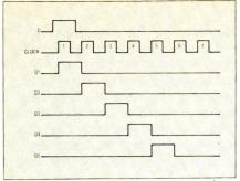
Fig. 2 The progression of a single bit of information through a serial in, serial out shift register.
