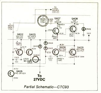
18ohm fixed resistor which may also overheat. Possible cause: Open top driver transistor base bias return resistor (220k-ohm  $\frac{1}{2}$  W 5%—R3117 in CTC 87, 88, 96, 97; R448 in CTC 93). If this resistor is okay, check for open printed circuit or components in the top driver, top output circuitry. When the top driver/top output is not operational, the retrace switch may be biased in such a manner that it attempts to supply current for top vertical deflection.
