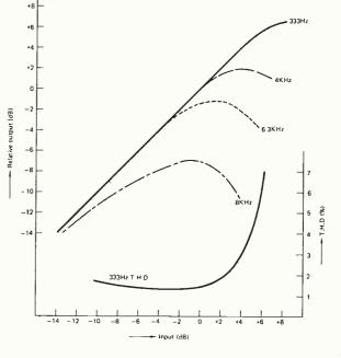
Fig. 5 Relative input and output distortion characteristics of cassette tapes
