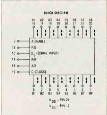
Fig. 12 The 4034 is a bidirectional register used to interface various buses. It may be programmed using four control lines.
