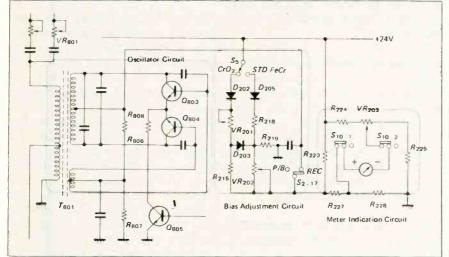
Fig. 9 The bias adjustment circuit in the CT-700
