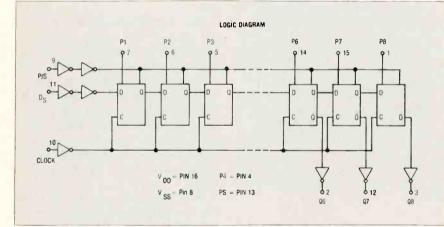
Fig. 10 The difference between the 4014 and 4021 is that one is a synchronous load device while the other serves as an immediate load.
