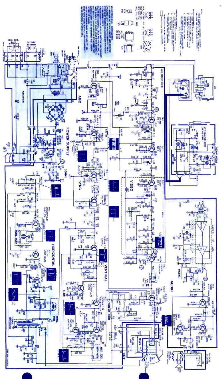
1814. B&W TV Chassis TX-493 COMPLETE MANUFACTURER'S CIRCUIT DIAGRAMS
