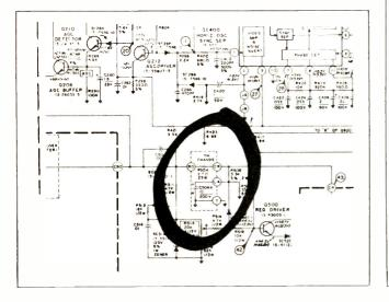
E21, Excessive high voltage—B+ rises to shut down level. Possible cause: Open C506A
