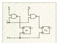
Fig. 3 The "parallel" entry shift register.
