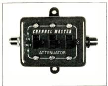
Fig. 2 A typical step attenuator–0 to 21dB in 3dB steps.
