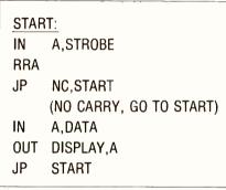
Fig 3-This simple keyboard routine demonstrates the basic principal of the 'wait loop.' The value of the bit indicating a keystroke is continuously tested until it is high, then the data is read and displayed.
