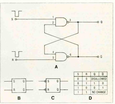
Fig. 1 - NAND-logic RS flip-flop, A) Circuit using TTL 7400 gates, B) Schematic symbol sometimes used, C) Alternate schematic symbol, D) Truth table.
