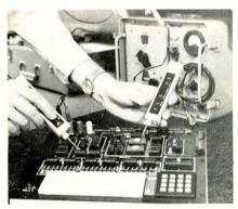
Fig. 12 - E&L Instruments MMD-1 trainer and Continental Specialties PL-2 logic test probe in operation.
