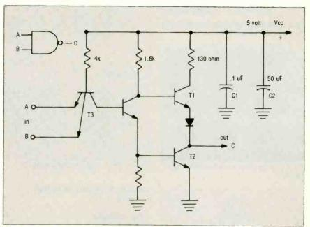
Fig. 7 - Typical TTL gate circuit and filter capacitors.
