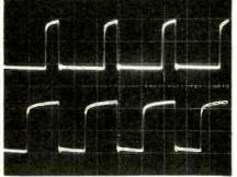
Fig. 4 - Timing pulses of a two phase clock system.
