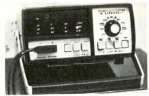
Fig. 3 - The DMM of the "future," Sencore's DVM56 "Microranger." This unit is microprocessor automated with non-blinking, LED readout; dcV to 10KV capacity; non-blinking peak and null with range hold; full AcV capability including PP, average, true RMS, or dB readings. Scheduled for Fall introduction. Circle no. 153.
