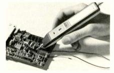
existing low state to high or high state to low. It is compatible with DTL, TTL, RTL and CMOS logic circuits. Operating power is supplied by the circuit under test. The net price is \$80.
