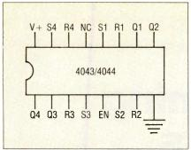
Fig. 5 - Pinouts for CMOS 4043 and 4044 quad RS flip-flop ICs.
