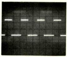
Fig. 8 - Normal TTL gate pulses.
