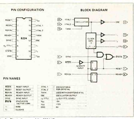
Fig. 6 - Block diagram of the 8224 IC.
