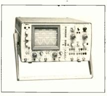
The DM3010 add-on DMM when used with the scope—it can be used independently—offers increased accuracy in measuring amplitude, time and frequency. The cost of of the OS3500 complete with probes is \$1995; the price of the DM3010 is \$360.
