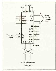
Fig. 5 - Block diagram of INTEL'S 8080A IC with data and address bus.
