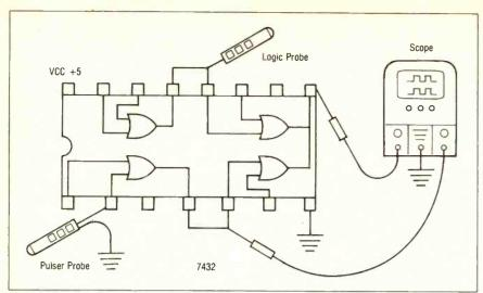
Fig. 13 - Set up for using pulser and logic probes plus a scope for monitoring several gate actions simultaneously.
