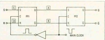
Fig. 4 - Master-slave flip-flop.
