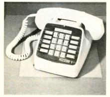
*Electronics Corporation.* The new telephone is a repertory dial telephone known as Access I. It can be programmed in seconds to remember nine frequently called or emergency numbers and automatically will remember the last number dialed manually. By depressing just two buttons, any of the stored numbers will be dialed automatically.
