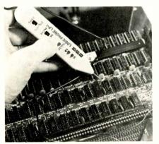
Fig. 11 - Logic probe being used to check ROM ICs.
