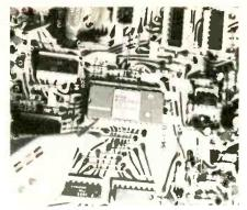
Fig. 3 - A GE EIC20 tuning control chip being checked with a log probe.
