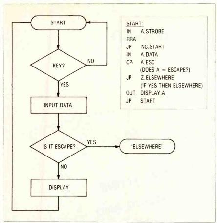
Fig 5-The improved keyboard routine (with its associated flowchart) allows exit upon depression of the ESCAPE KEY. Note that after the "compare" instruction, which checks the Accumulator against the value 1B, the ZERO Flag is set to indicate an "equals" condition. The next statement directs the processor to go ELSEWHERE in this case.
