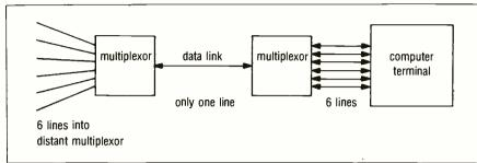
Fig. 3-A block diagram of a multiplexor data transmission system.
