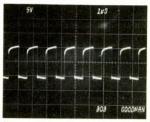
Fig. 2 - Clean clock pulse with properly grounded probe.
