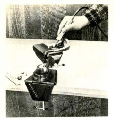
a work piece. Machined slide rods assure parallel jaw alignment and equalized work pressure.
