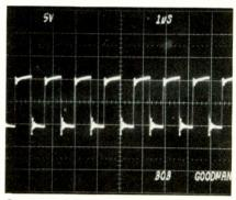
Fig. 1 - Distorted clock pulse due to improperly grounded scope probe shield.
