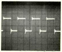
Fig. 9 - Spikes due to open filter capacitors.
