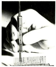
The compact, inexpensive WSU-2224 tool, from OK Machine and Tool, wraps, unwraps and strips wire, thanks to a unique built-in stripping blade. Designed for use with 22-24 AWG (0.65-0.50mm) wire on standard .030  $\times$  .060 in. (0.76  $\times$  1.52mm) and .045 in (1.44mm) square posts. Reportedly takes minutes to learn to use and makes connections in seconds without solder. Priced at \$12.75.
