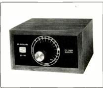
FM reception, it is stated it can be used also in suburban areas where only indoor antennas may be used. Specifications include an RF gain of  $35dB \pm 5dB$ ,
