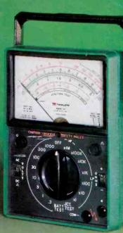
These VOM's have X-TRAT rugged construction that can take a 5 ft. drop onto a concrete floor! They're safety engineered throughout with an unusual diode and multiple fuse arrangement providing overload protection for all ranges. Single selector switch reduces errors, in fact, the 60's eliminate over 90% of costly repairs from VOM misuse.
