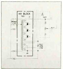
Fig. 6 Flyback transformer from Y-2 chassis.
