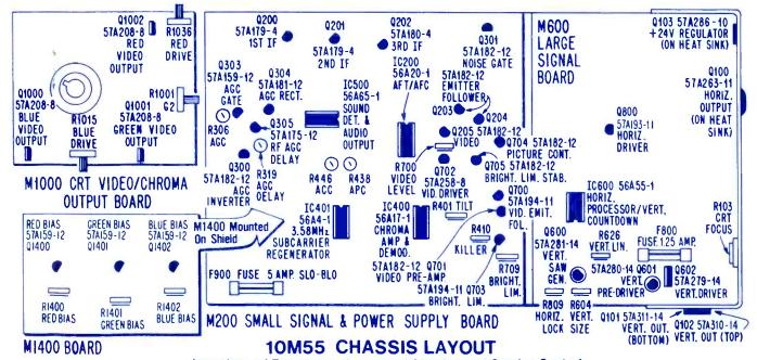
Locations of Transistors, Integrated Circuits, and Service Controls.
