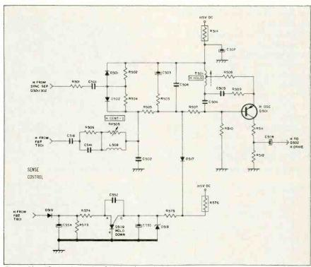
Fig. 5 Simplified schematic of high voltage hold down circuit.
