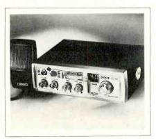
Pace has announced the early fall availability of a new domestically manufactured CB transceiver, the Model 8016. The manufacturer states that this radio uses the very latest state-of-the-art large-scale integration (LSI) semiconductor technology for high efficiency in a small space. Reportedly it far exceeds Federal Communications Commission
