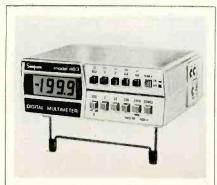
Simpson Electric Company has recently introduced a compact, portable, digital multimeter, the Model 463, a 3½ digit LCD instrument with 26 ranges. The low current LCD readout and all LSI circuitry permit up to 200 hours of continuous operation on a 9V alkaline "transistor" battery. The Model 463 has 5 dc volt
