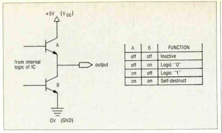
Fig. 2-Tri-state logic devices. Normal TTL IC's, to produce two-state output, always have transistor A or B of the totem-pole output ON. Tri-state devices allow Party-line use of data bus by allowing both transistors to be off, making the device logically disappear.
