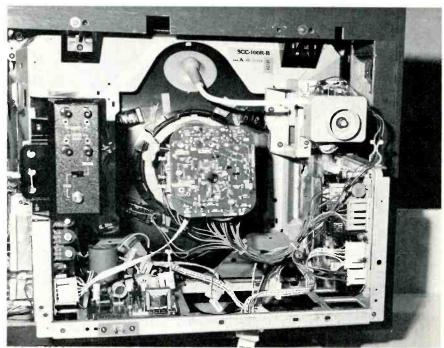
Fig. 1 The Sony "I2" chassis with one board removed. (Courtesy Sony Corporation of America)
