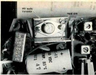
Fig. 7-In some table model radios a large single power output transistor is found bolted to a small heat sink.
