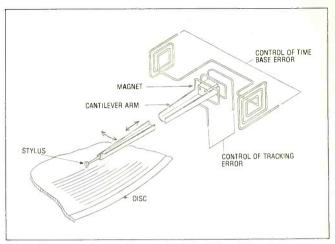
Fig. 2 Diagram showing the electro tracking system.
