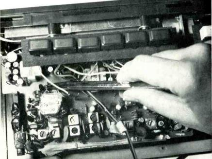
Fig. 10-The FM oscillator transistor may be located next to a couple of air-wound selfsupporting coils and close to the variable tuning capacitor.
