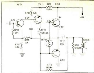
Fig. 9-A schematic of a transformerless sound output stage with normal transistor voltages.
