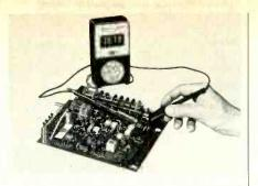
cept for the ½ digit. Ranges of the Model 3400 are 200 mv to 500 v ac and dc in 5 ranges, 2 to 2000 ma ac and dc current in 4 ranges and 200 ohms to 20 Megohms in 6 ranges. The ohmmeter features high and low power ohms ranges for semi-conductor circuit resistance measurements. The Model 3400's price is \$140 with test probes, battery, instruction book and 1 year warranty.
