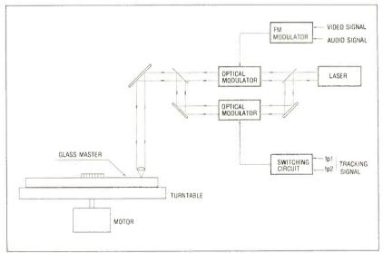
Fig. 3 Information and tracking signals are recorded optically and are carried to their destination via split beam laser.
