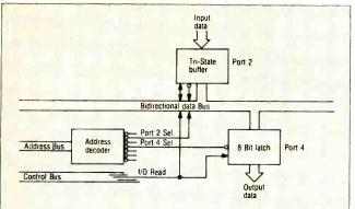
Fig. 4-Typical input/output logic of a system, showing one buffered input port and one latched output port. Address decoder and command line from the Control Bus govern the data flow, injecting or extracting data into or out of the data bus at the proper time.
