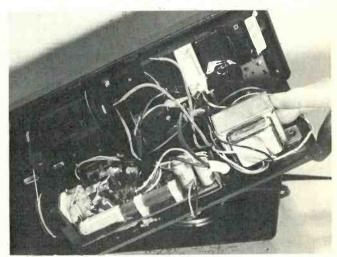
Fig. 5-Some table and portable receivers have a power transformer to operate the radio and digital clock circuits (Dyn model DS4555).
