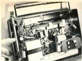
Fig. 6-A tunetable squealing noise was heard across the entire band in a Magnavox IR-1201 3-band radio. The finger points at the defective decoupling capacitor.
