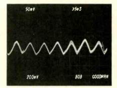
Fig. 6-Ripple voltage found on +23 volt supply line that should be a smooth scope trace.
