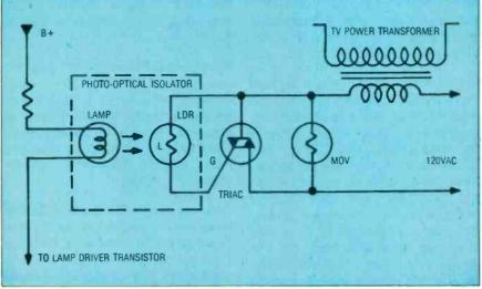
Fig. 7-Zenith on/off remote control circuit.
