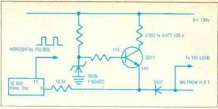
Fig. 2-Sony's "kick" start circuit which provides start up current for the horizontal oscillator.
