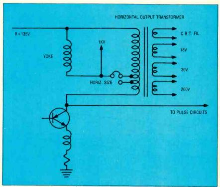
Fig. 3-Simplified DC circuitry of the horizontal output transformer which provides scan derived voltages for the filament, 18, 30, and 200 regulated supplies.
