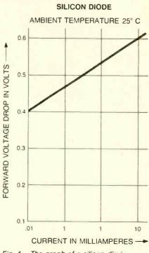
Fig. 1 - The graph of a silicon diode.
