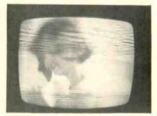
Fig. 3-Top and bottom criss-cross pattern.
