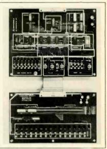
stration unit. Based on the company's recently introduced single-bit microprocessor-the MC14500B ICU-the system has 15 inputs and 16 outputs, and incorporates a RAM capable of holding 128 ICU program instructions. The user is able to examine or change the contents of any memory location and has the option of single stepping or running his program. The system operates from a 5-volt power supply, and is priced at \$295.
