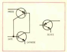
Flg. 1-Schematic representations of the Gate Controlled Switch.
