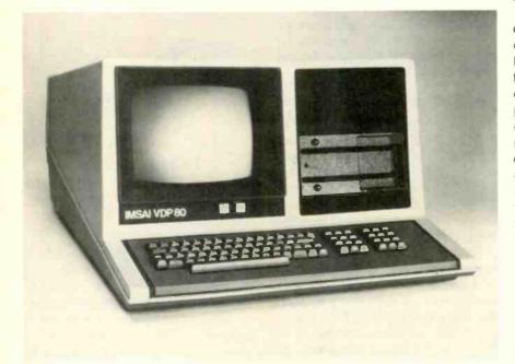
Fig. 5-Complete, self-contained, desk-top computer system intended for small business applications (courtesy Imsai Mfg. Corp.).
