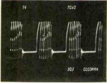
Fig. 2–Abnormal scope trace found at base of Q202 caused by open filter capacitor.
