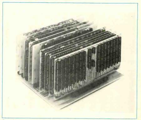
Fig. 4-Most computers use a mother board Interconnection bus with plug-in cards (courtesy, The Digital Group, Inc.).
