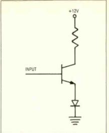
Fig. 4 → This signal expansion clrcuit behaves in a reverse manner from an AGC system. Diode resistance falls as input signal Increases (emitter current increases).
