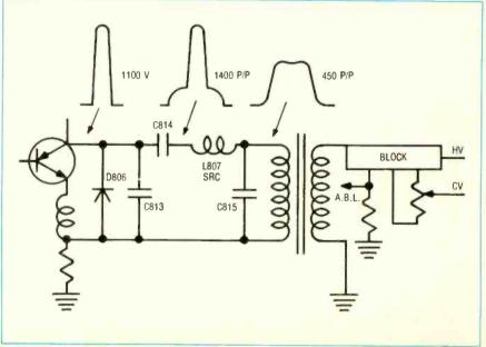
Fig. 4.-A. C. Circuits retrace pulse.
