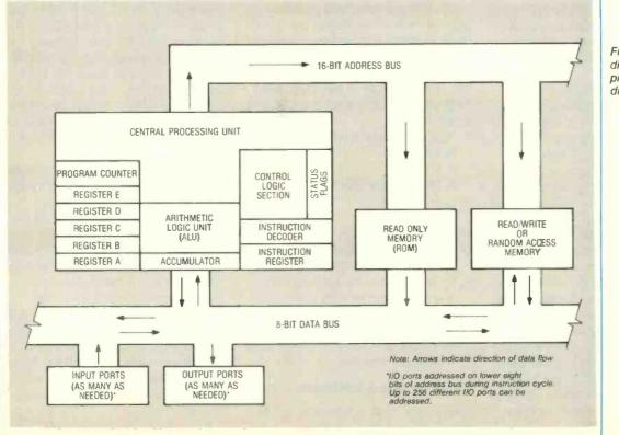
Fig. 6–Block diagram of a typical programmable digital computer.
