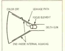
Fig. 8–Picture tube diagram illustrating second anode internal leakage to focus element.
