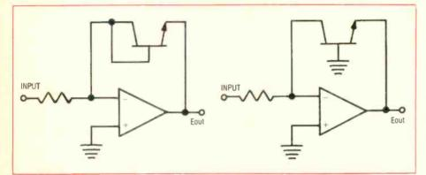
Fig. 3 - (A) Transistor connected as a diode. (B) Used as a transconductance device in the feedback path.
