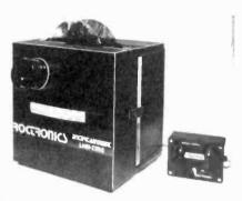
Discs are inserted into two slots on the projector top and their speeds and direction are varied to achieve the desired effect. The standard lens shows horizontal motion and the interchangeable kaleidoscope lens creates six-sided symmetry. The projector is portable, weighs 12 pounds, is a nine inch cube, has a carry handle, and uses a standard 300 watt quartz lamp. It sells at retail for \$500.
