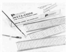
and application to the wire. Available in all popular legends, the markers are 1<sup>1</sup>/<sub>2</sub> inches long and will wrap around all wires up to 3% inches outside diameter. Material is vinyl impregnated cloth suitable for use in temperature ranges from  $-40^{\circ}$ F to  $250^{\circ}$ F.
