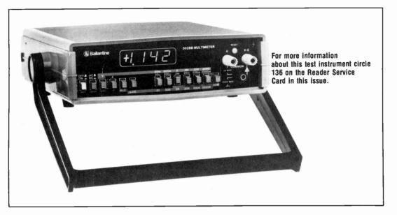
■ Ballantine Laboratories have just introduced a new portable rms responding digital multimeter with a sensitivity of 10 mV Full Scale and it is their claim that it is the only 3½ digit DMM to have 10 uV resolution and the capability to measure 10 milliohms.
