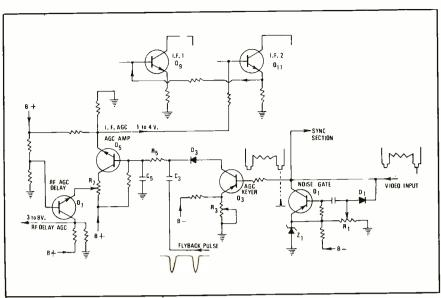
Fig. 3-A typical all-solid-state keyed AGC system.
