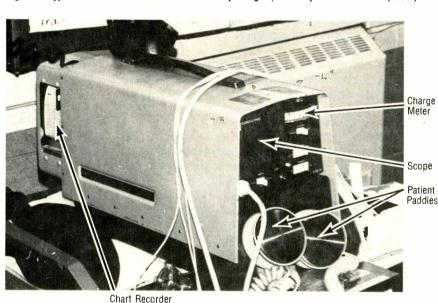
Fig. 3—A battery-operated portable defibrillator.
