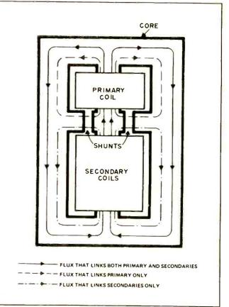
Fig. 1-Constant-voltage transformer construction.
