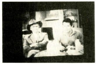
Fig 8-Small picture caused by open C1207.
