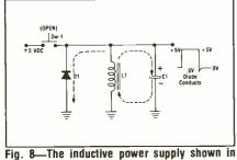
Fig. 7 with the suppressing diode added to the circuit in the 'off' position.
