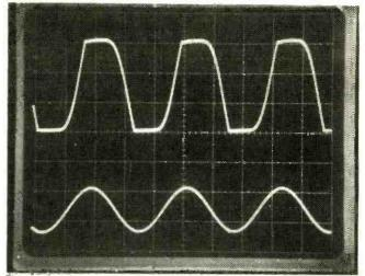
Fig. 3—Scope traces for normal line voltage.
