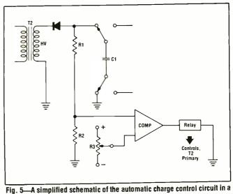
Fig. 4-A simplified schematic of a typical defibrillator.
