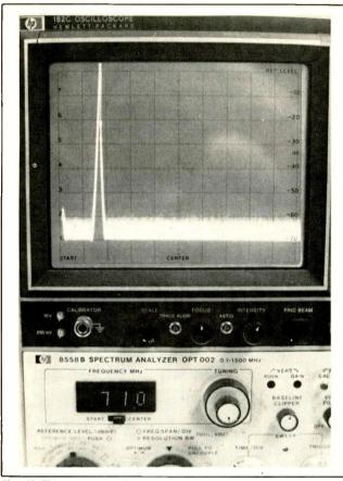
Fig. 1—The trace appearing on a spectrum analyzer shows white noise along the frequency base line. Broad-band noise appears like grass, as if one were looking at a cross-section of thick turf. On a TV picture tube, it appears as snow. From a loudspeaker, it is a frying noise.
