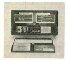
Rear view of Dana Model 2100A Digital VOM with cover of battery/fuse compartment removed. Single non-chargeable 9-volt battery provides one year of operation.
