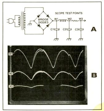
Fig. 26—Three-section filter system.
