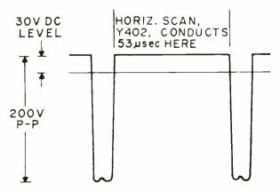
Fig. 14—Horizontal retrace pulses used in scan rectification.
