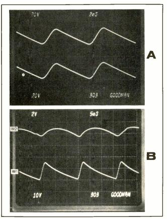
Fig. 25-Waveforms indicate a shorted choke.
