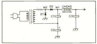
Fig. 21-Full-wave doubler circuit.
