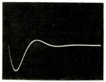
Fig. 7—A typical waveform taken across a 50 ohm dummy load in a properly operating defibrillator.
