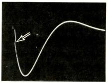
Fig. 8—This is an expanded scope display of the left portion of the waveform in Fig. 7. Arrow points to the "glitch" caused by a defective HV relay.
