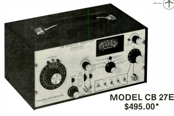
Low-cost, rugged, portable instrument for accurately checking, trouble shooting and aligning Citizens Band Transceivers operating in any of 40 Channels presently assigned.
