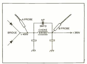
Fig. 23-Dual-trace connections for checking the filter system.
