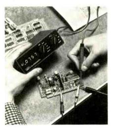
high-resolution unit offering 4½ digit resolution on all parameters. It is convertible for bench use with an optional bench stand, and features 10 microvolt sensitivity DC and AC and basic oneyear accuracy of  $\pm 0.05\%$  of input. Most logic components in the Model 248 are contained in a single LSI chip. It has only two controls, function and range. Priced at \$345.
