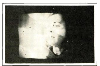
Fig. 11-Slight picture bend due to shorted choke.
