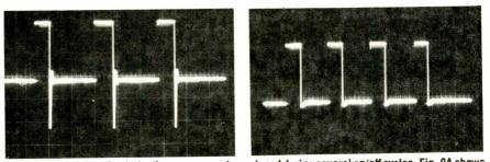
Fig. 9—Waveforms of an inductive power supply produced during several on/off cycles. Fig. 9A shows the negative spike produced when the suppressing diode is open or missing. Fig. 9B was produced by a power supply circuit with a properly operating suppressor diode.
