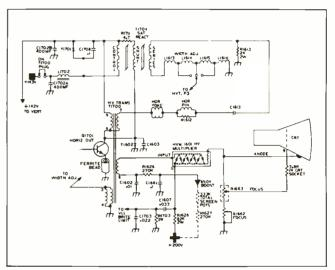
Fig. 9-GE MC chassis filter and high-voltage circuits.
