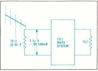
Fig. 2—Diagram of 75-ohm matched impedance MATV system showing that theoretical-minimum thermal-noise voltage is 1.1  $\mu$ V/ch (-59.1 dBmV) at room temperature.
