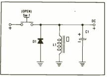
Fig. 6—Diagram of an inductive power supply circuit that could be a solenoid, relay coil, flyback coil, or deflection yoke.
