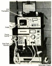
Fig. 1-A typical defibrillator resuscitation cart.
