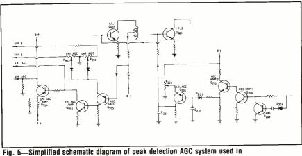
Fig. 5—Simplified schematic diagram of peak detection AGC system used in some Sony color TV receivers.
