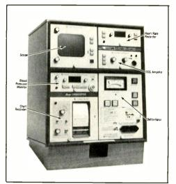
Fig.2—A bedside defibrillator and monitoring package. (courtesy of American Optical)
