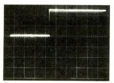
Fig. 3—A normal rising waveform of a positive power supply that is mostly resistive.
