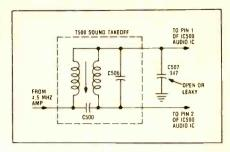
**CAUSE:** Open or leaky capacitor C507, which is connected to Pin 1 of the audio IC, IC500.
