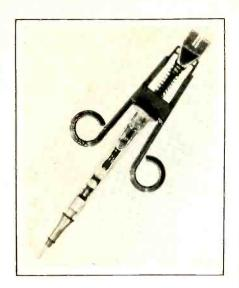
vice features a precision width, high mass heating head for maximum pin contact and heat transfer. All of the IC pins are heated uniformly so the IC may be quickly removed the instant the solder becomes molten. The manufacturer says heat damage to the board is minimal. After the holes are desoldered, a new component may be directly soldered in place. The extractor includes heat-resistant plastic forceps and stainless steel tongs which grip the IC for fast removal.
