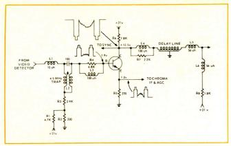
Fig. 2—Schematic diagram of the 1st video amplifier stage of the video amplifier section shown in Fig. 1.
