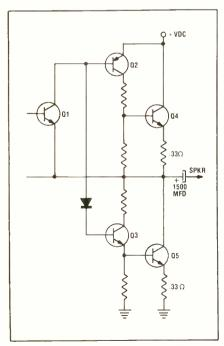
Fig. 5—Quasi-complementary amplifier uses identical matched output transistors but has complementary drivers. These lower power transistors are sometimes easier to source out in low-power complementary pairs.
