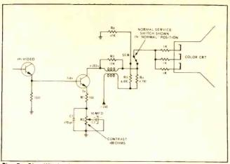
Fig. 5—Simplified schematic diagram of the video output stage and CRT cathode drive circuit.
