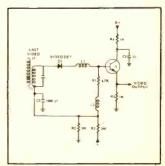
Fig. 3—Simplified schematic diagram of an emitter-follower type of 1st video amplifier which might be used in place of that in Fig. 2.
