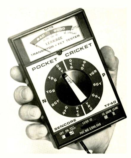
connected to the device.) Once a single 'good gain" position of the TEST switch is established, the device's leads can be physically identified by matching the element-to-test lead color code of that TEST switch position to the corresponding color-coded test leads connected to the device's elements.
