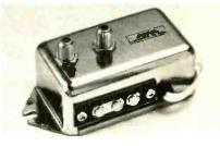
introduced by *AVA Electronics Corporation*. The device features a bandwidth of 50-900 MHz and has an output capability up to 30 dB. The power source is a 117V AC-60 Hz isolated transformer. The model features built-in lightning protection. It lists for \$37.95.
