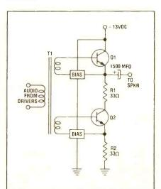
Fig. 3—Totem-pole push-pull power amplifier uses identical power transistors driven by a special transformer with two secondaries which drive the bases out of phase.
