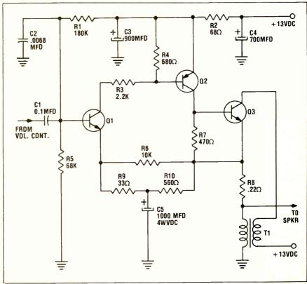
Fig. 2—Bendix version of the NPN silicon Class-A power amplifier. Similar circuitry also is used by Philco (now Aeronutronics-Ford) and others. Transistor Q3 is usually a P-66 plastic power transistor.
