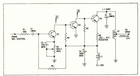
Fig. 1—Classic PNP Class-A power amplifier used in auto radios since the early '60s. Transistor Q3 is usually a germanium type such as the Delco DS-501 or DS-503 or the Motorola 2N176.
