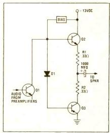
Fig. 4—Complementary symmetry push-pull power amplifier depends upon the "opposite" characteristics of matched PNP and NPN power transistors.
