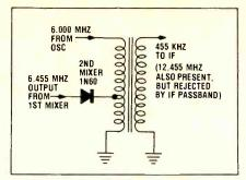
Fig. 2—Example of diode-equipped mixer circuit used in some CB transceivers.
