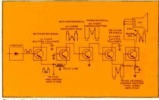
Fig. 1—Simplified block diagram of a five-stage color TV video amplifier section.
