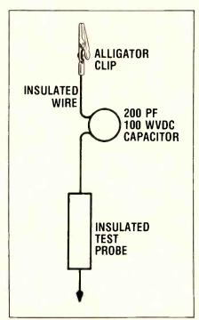
Fig. 3-Simple, do-it-yourself signal-injection probe. Usage is explained in the text.
