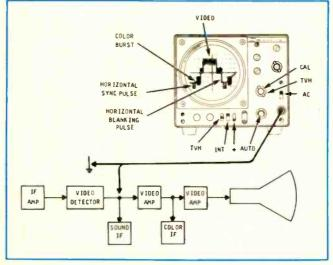
Fig. 1—Test setup for observing two complete horizontal scan lines of the Fig. 2—Test setup for observing two complete vertical fields of the composcomposite TV signal. (Courtesy of B&K-Precision.)
