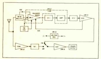
Fig. 1—Block diagram of 1976 Delco Chevette
