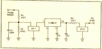
Fig. 4—FM IF amplifier section of DM-37 IC in the Chevette radio. CF1 and CF2 are ceramic piezoelectric filters.
