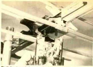
Plastic housing protects preamp circuits from wind, rain and dirt. A rubber boot seals the opening where the cable enters the case.
