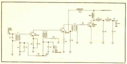
Fig. 1—A composite version of the circuitry typically found in the RF amplifier sections of today's CB transceivers.
