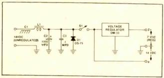
Fig. 5—Simplified schematic diagram of the Chevette radio's power supply. DM-33 is a new three-terminal voltage regulator device.
