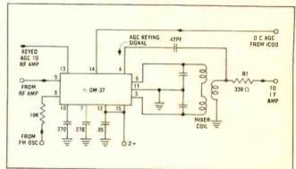
Fig. 3—FM balanced mixer section of the DM-37 IC used in the Chevette radio.
