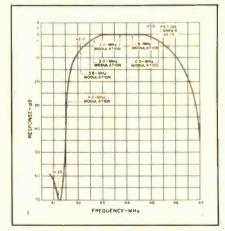
Fig. 8—Typical color TV video IF response curve. (Courtesy of B&K-Precision.)
