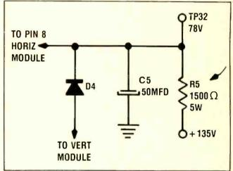
CAUSE: If cause is traced to a defect on the horizontal module or a defective horizontal output transistor Q1, always check the voltage at TP32 after replacing either the module or Q1. The voltage at TP32 should be about 78 volts. If it is significantly higher, the value of R5 (1500 ohms, 5W) probably has decreased, in which case R5 should be replaced to prevent repeated failure of the horizontal module or transistor Q1.
