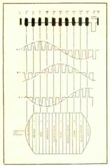
Fig. 15—Top waveform here is the input of the color bandpass amp section (point 1 in Fig. 16), with a keyed color bar signal applied to the input of the receiver. The three other waveforms are those at the outputs of the color difference amplifiers. The resultant pattern produced on the screen is shown at the bottom.
