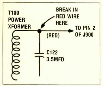
CAUSE: Break in small red wire in power transformer circuit at the point where capacitor C122 connects to it. This red wire, which is dressed in a bundle of other wires, connects C122 to pin 2 of J900. A break in this wire causes the regulated 130V B+ supply to decrease below 130V as the brightness level is increased.
