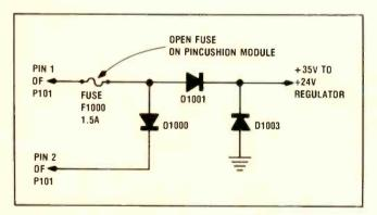
CAUSE: Open fuse F1000 (1.5A) on A8954-3 pincushion module. Opening of this fuse eliminates the 33- and 24-volt supplies, disabling the vertical sweep and sound sections. In some cases there is no apparent cause for the opening of fuse F1000 (Admiral part No. 84-A4-7), and replacing it restores both vertical sweep and sound. In other documented cases involving earlier runs of the M10 Chas-
