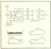
Fig. 16—Block diagram of a typical chroma section which shows key waveform observation points. Four key waveforms are shown below the block diagram.
