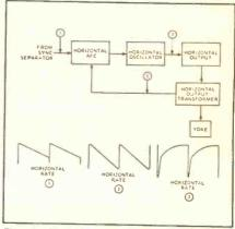
Fig. 14—Block diagram of typical horizontal deflection system, and associated waveforms.
