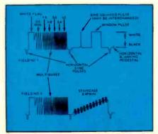
Flg. 5—Composition and content of the vertical interval test signal (VITS). Shown here are vertical fields 1 and 2. (Courtesy of B&K-Precision.)
