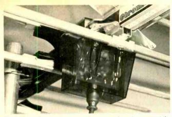
Metal clips on the circuit boards of the preamp shown here connect the preamp input directly to the antenna phasing lines, thereby providing optimum impedance matching and minimum loss.
