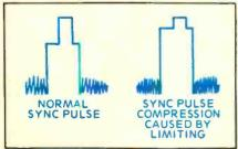
Fig. 4—A defect which shifts the operating point of the video IF amps can cause horizontal sync compression, as shown here. (Courtesy of B&K-Precision.)
