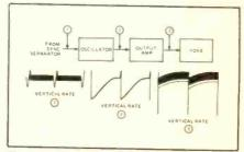
Fig. 13—Block diagram of vertical deflection system and associated waveforms.
