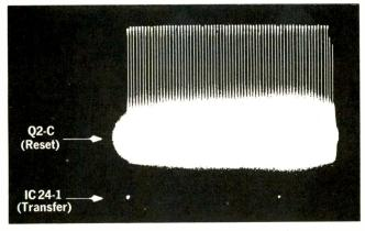
Fig. 9—There are a hundred reset pulses for every transfer pulse.
