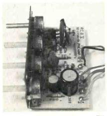
The DETAIL, BRIGHTNESS, CONTRAST and VER-TICAL controls are mounted on a separate video preamp board.
