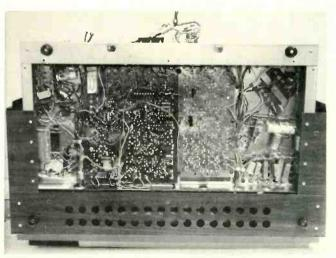
After removing a panel the complete underside of the chassis is exposed, making solder connections very accessible.
