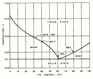
Melting Temperatures of Various Solder Alloys
