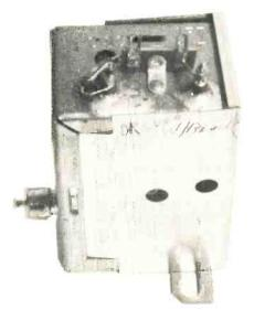
The AFT module is coupled to the IF module with a phono-type jack connector and is mounted on the top of the main chassis.
