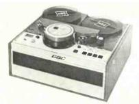
stop motion, solenoid operated controls, auto-cycling and automatic gain control. Tapes made on the unit can be played back on any standard recorder. GBC.
