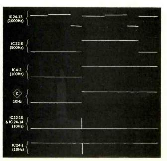
Fig. 8—Even though the signal frequencies range from 1kHz to 10Hz, there is still a definite timing relationship.
