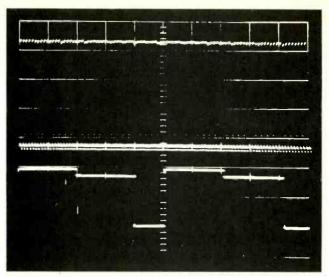
Fig. 6—Comparing the 1kHz signal applied to Inverter B (upper trace) with the 10Hz applied to capacitors C11 and C12 (lower trace).
