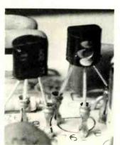
The transistors are mounted in sockets to shorten service time, if removal is necessary.
