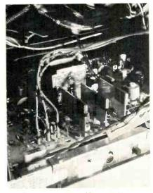
The blue, red and green video output transistors are plugged into the chassis and employ large heat sinks. Also shown are the ground pins to disable the color guns for purity adjustments.
