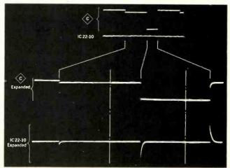
Fig. 4—Differentiated pulses from the 10Hz signal are used for resetting the flip-flop circuit.
