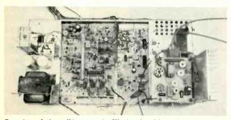
Top view of the solid-state color-TV chassis with road-mapped circuit boards to simplify identification of components.
