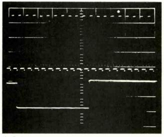
Fig. 7—By increasing the sweep rate by  $\times 5,$  more detail of the 1kHz and 10Hz signals can be observed.
