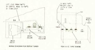
resistor is wired in series with the ground (black) lead of the VOLUME control. Mount the resistor as shown.
