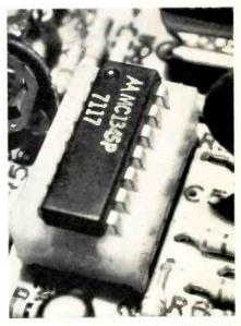
The integrated circuits are plugged into sockets for ease of removal when using the substitution method of servicing.
