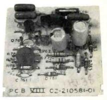
The auto-saturation printed-circuit board employs edge connectors and plugs into a socket on the main small signal printed-circuit board.
