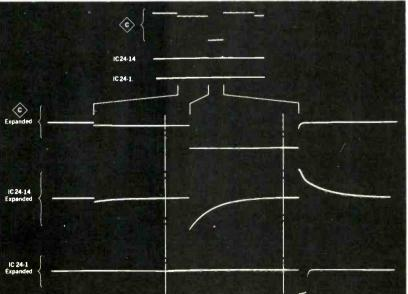
Fig. 5— Differentiated pulses from the 10Hz signal are used for producing the transfer signal.
