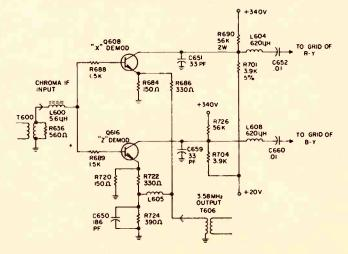
Fig. 4 - Schematic showing the X and Z demodulators.
