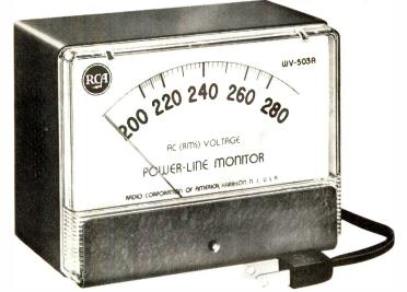
**The RCA WV-503A** 240-Volt Power Line Monitor is the big brother of the WV-120A. At a glance, it provides a continuous, accurate indication of the AC line voltage from 200 to 280 volts. Used in conjunction with a variable isolation transformer, it is an invaluable aid in selecting line voltages for TV servicing, test equipment calibration and the operation of electronic equipment that requires a known line voltage supply. ONLY \$18.50.\*
