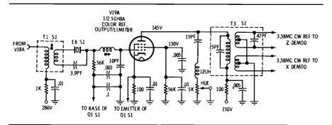
to the two demodulators in such a phase as to detect "X" signals at one, and "Z" signals at the other.
