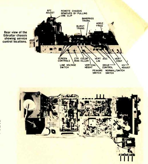
Top view of chassis showing the plugability concept carried throughout the entire chassis.
