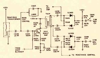
Fig. 3 – The burst amplifier and phase detector circuits.
