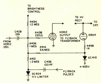
Fig. 7 - Schematic of the HV protection circuits.
