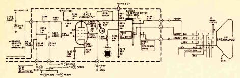
Fig. 1 - The brightness control and dc restoration circuit.
