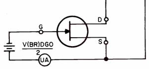
Maximum voltages specified by the manufacturer indi cate lowest voltages that may be applied between element that will lead to device breakdown.
