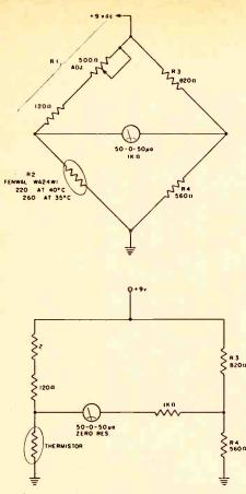
Fig. 5A – A Wheatstone bridge circuit as we might see it in an industrial schematic.
