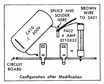
wire, C401 pigtail and F402 pigtail together as shown and solder. Clip off any excess wire at joint and dress the splice outward to make sure that there is no possibility of splice touching vertical output transformer.
