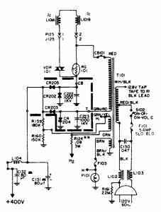
Never attempt this on any KD chassis since the tap on the KD chassis transformer primary is for Insta-View and not high line voltage.
