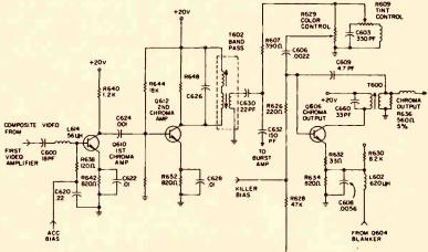
Fig. 2 – The chroma IF amplifier circuit shown attenuates low frequency video and passes frequencies in the chroma IF band.
