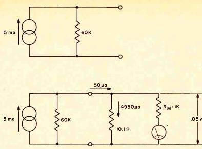
Fig. 7A - Norton equivalent of microammeter circuit.
