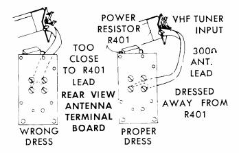
Refer to the drawing and dress the  $300\Omega$  lead well away from R401, as shown, before the back of the receiver is reassembled.
