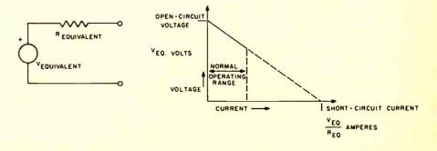
Fig. 1 - A Thevenin equivalent circuit and its load line.
