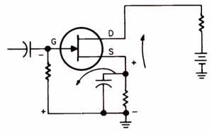
The illustration shows the connections to make gate leakage tests. The resistance in this circuit will be very large allowing only nanoamperes or microamps current flow. This is true especially of the IGFET's. Junction type resistances are very temperature-sensitive, similar to semiconductor diodes.
