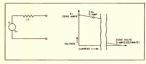
Fig. 4B – The same circuit redrawn to emphasize the relations between voltage, resistance and unknown load.
