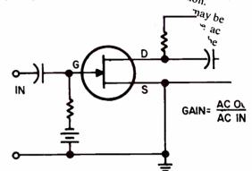
measured by connecting an amplier and comparing signal out to signal in. Shown in typical fixed and self-biasing arrangement.
