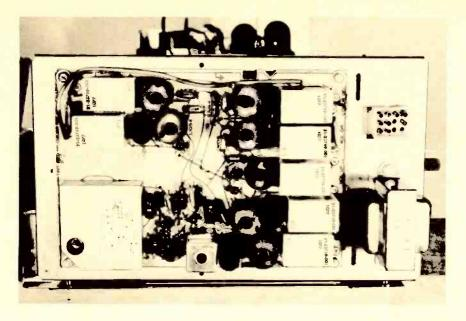
The remote control receiver chassis with plug connectors are easily removed by removing one clip on the mount.
