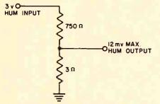
10-Thevenin equivalent circuit for Fig. estimating maximum possible hum.
