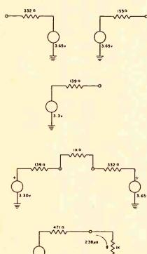
Fig. 6A - Thevenin equivalent of RH voltage divider.
