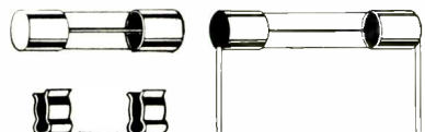
Fig. 1 — Clip-in and solder-in type fuses are among the fuses approved by UL.
