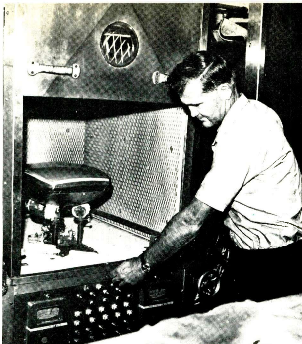
A tube is placed in the Windsor oven for baking. The temperature will be brought up to 240° F and evacuate the tube. This cycle normally takes two and one-half hours for a color tube.
