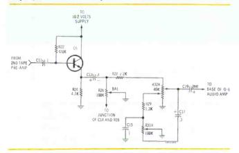
circuit of the audio predriver, Q6. The forward bias for the emitter follower is furnished by Q5. The output of Q5 is developed across load resistor R24. Audio to the volume control is coupled by C13.
