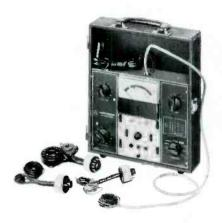
Have you ever checked a color CRT that read "good," but actually the tube was bad? Now you can check for that hidden problem—internal high voltage leakage —at actual operating voltages ..., right in the customer's home. The CRT Commander, Model 857, can test every performance characteristic of a picture tube. Black and white or color.
