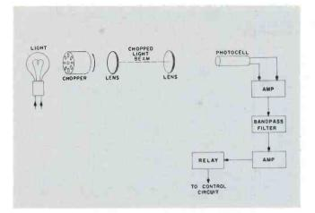
Fig. 3—Mechanical chopper modulates light beam which passes through bandpass amplifier to prevent receiver from
