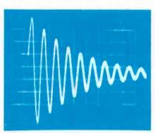
Fig. 5 — Proper ringing waveform as seen on scope.
