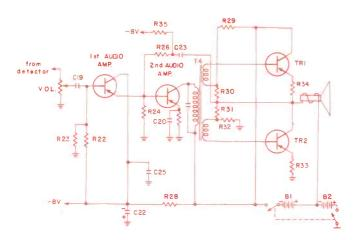
Fig. 1—Class B, solid-state audio amplifier. Courtesy Westinghouse.
