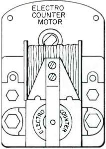
replace "leaf switch" S1002, stock number 115497. Condition "B." Where CR1202 diode has failed and an Electro Counter motor is used: (1) Add  $10 \,\mu$  f capacitor C1201 — if it is missing, stock number 118832. (2) *Continued on page 89*
