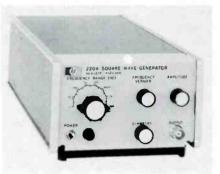
trolled oscillator. Source impedance is  $50 \Omega$ . This, it is said, preserves the clean waveshape by absorbing reflections from impedance mismatches on the output cable. The model 220A measures 5 1/3 x 3-7/16 x 115/sin. Price \$195. Hewlett-Packard.
