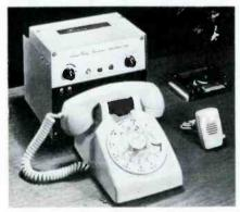
ed. The unit employs an endless tape contained in a snap-in cartridge onto which both incoming and outgoing messages may be recorded, according to the maker. It is said the unit is not wired into telephone company lines. It carries a one-year warranty policy. Minatronics.
