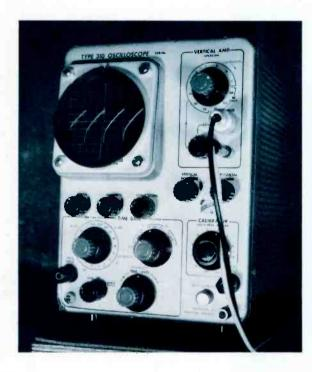
Fig. 4 --- Tektronix type 310 single-channel triggered scope.
