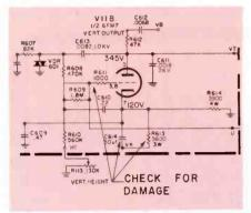
vertical tube fails. The extent and nature of the secondary damage will vary, depending on the nature of the tube failure.
