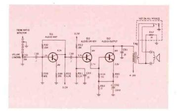
Fig. 2—Audio amplifier system used in Motorola's TS400 TV chassis.
