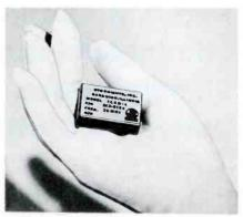
PC board mounting, the model JKTC-XO-4 is available with any output frequency between 6 and 20MHz over a temperature range of  $-55^{\circ}$ C to  $+85^{\circ}$ C at stability of 1 x  $10^{-5}$ , the manufacturer says. The temperature compensating circuit is said to eliminate the need for a crystal oven — reducing warm-up time to zero and lowering input power to 100mw maximum @12vdc. Size is 1.5 x 1.0 x.40in. max. CTS Knights.
