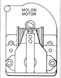
Where there is a tendency to skip a VHF channel or jam and a Molon motor is used, replace motor with Electro Counter motor stock number 119680. Amphenol's new 857 tests for second anode leakage to CRT gun structure.
