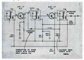
In solid-state circuitry, this becomes more difficult since the transistor is basically a "sharp cut-off" device. Many radio receivers use the overload diode to accomplish a measure of "AGC."
