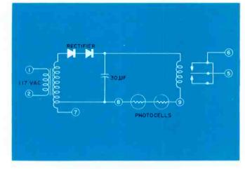
Fig. 4—A system which employs a sensitive balanced relay.
