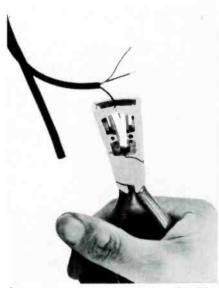
justment by the user, it is said. The stripper has 11 narrow cutting blades in each jaw. Each blade "floats" in its own spring mounting, so they close around the wire in a circle as the handle is squeezed. Cutting tension is provided entirely by the spring action in the blades—not by the amount of squeeze given the handle. Telvac.
