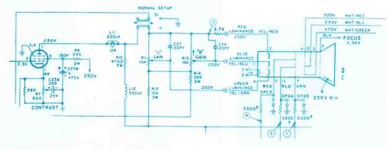
Fig. 8—Video section of Zenith 25MC36Z showing spark gaps 3, 4 and 5; C25A and B and CRT bias control, R15.
