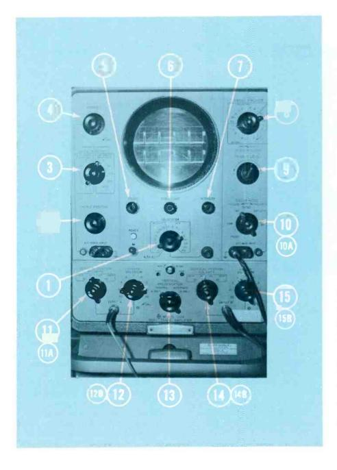
choice of electronic switching at about a 100kHz rate of electronic switching on alternate sweeps. ("Sweep" refers to the horizontal deflection of the trace.) You can also choose a highgain single-trace, a fast rise or a differential-input plugin unit. The differential unit provides the difference between two vertical-input signals, rejecting the common-mode signal.
