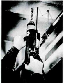
ducts and lighting fixtures. The No. 816 hammer/drill features an exclusive insulated shift collar for easy and safe conversion from hammer to drill action. Black & Decker.
