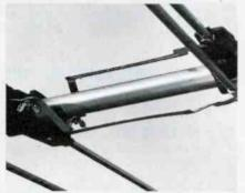
Balanced phasing lines, of rugged aluminum, stay in shape.
