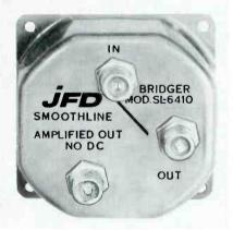
MHz, 470 to 890MHz; impedance 75  $\Omega$ ; isolation between through line and tap, 35db; through-line loss less than 1.0db; output gain, VHF, 1db UHF, -1.5db; tilt control range, VHF, 5.5db; dimensions; 2 5/16 x 2-5/16 x 1½in. List price is \$37.50. JFD.
