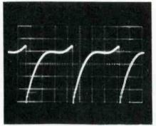
Fig. 2 — Misshaped drive pulse caused by waveshaping network (C603 and R602) being out of circuit. Also, C604 was defective.
