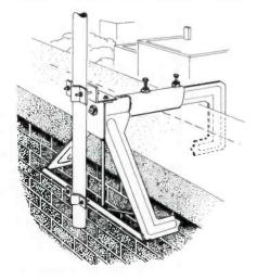
arc welded for extra strength and rigidity and hot-dip galvanized for corrosion resistance. No holes are necessary in parapet or roof. The mount is adjustable to accommodate parapet walls from 4 to 13in. thick. South River.
