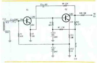
sistor, Q1, is a NPN silicon type, specially selected for low noise applications. Direct coupling between the collector of Q1 and the base of Q2 is used for better frequency response. The feedback network, consisting of C3 and R9, is used for tone shaping because of characteristics in the tape and playback head.
