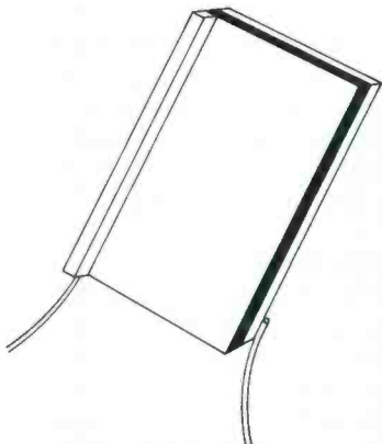
Fig. 3 — The substrate of a front-wall photovoltaic cell collects a positive charge when exposed to light.
