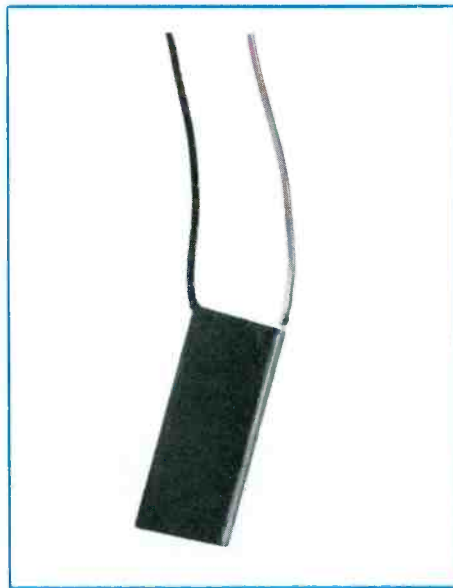
Fig. 1 — A series of these photovoltaic cells can be used to supply the electrical power for a transistor radio.
