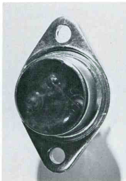
Fig. 11 — This phototransistor has a sufficient signal output to drive a relay without any additional amplification.
