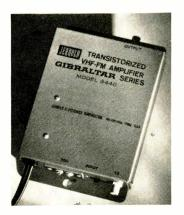
Heart of the system is the new solid-state GIBRALTAR amplifier. Low noise figure (less than 6 db) means GIBRALTAR works well even in weak-signal areas. High output capability (more than 150,000 microvolts) lets it work in very-strong-signal areas without overload. High gain (25 db avg. hi band; 23 db avg. lo band and FM), consistent performance and maintenance-free reliability make GIBRALTAR the ideal amplifier for every small VHF system you install.
