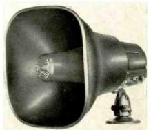
to 30w. Power, equalized to frequencies above horn cutoff, 40w. Frequency response, 225-14,000cps. Audio level, 125db measured 4 in. on axis at 30w input. Dispersion, 100 deg. Atlas.
