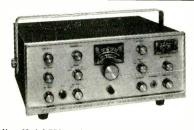
New Model 753 — The one and only SSB/AM/CW Tri-Band Transceiver Kit. 200 watts PEP on 80, 40 and 20 meters. Receiver offset tuning, built-in VOX, high level dynamic ALC. Unequalled performance, features and appearance. Sensationally priced at \$179.95 kit, \$299.95 wired.
