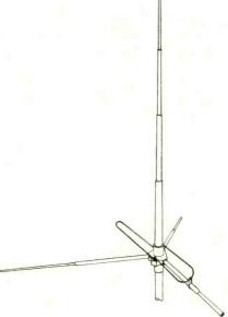
pattern, according to the announcement, is 360 deg circular. A coaxial female connector is incorporated into the weather-proof radial support assembly. VSWR is reported to be 1.5:1 or better and gain at 3.4 db over a quarter-wave ground plane. Mosley.
