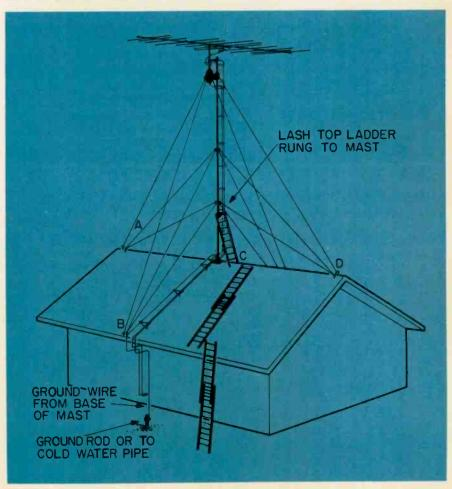
and guiding it with arm and shoulder. When the mast is vertical, lift and pull the base end away from the wall about 2 ft, allowing the mast to rest against the open bracket at the gable. Tie the rope to the base of the mast so it won't slip and go slack.
