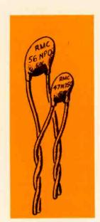
Fig. 1-A 44 pf N750 and 56 pf NPO capacitor are paralleled to obtain a total of 100 pf with TC of N330.
