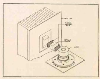
Cross-sectional diagram of new conduction cooling system designed by Amperex Electronic Corp.
