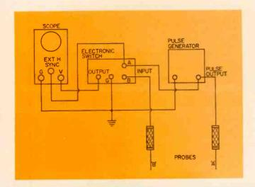
Fig. 5—Setup employing pulse generator, switch and scope.
