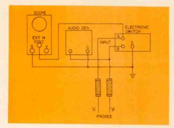
Fig. 3—Setup employing audio generator, switch and scope.
