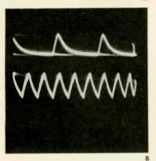
Fig. 2 (A)—Scope pattern indicating no defect in PC board. (B)—Trace indicated a defective circuit board in horizontal sync section of a color TV receiver.
