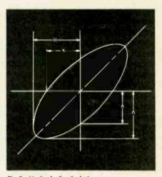
Fig.3—Method of calculating impedance from scope pattern. A slightly different arrangement can be used for calculating phase differences also.
