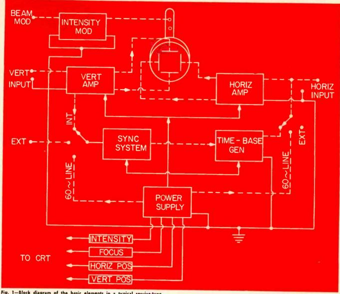
Fig. 1-Block diagram of the basic elements in a typical service-type
