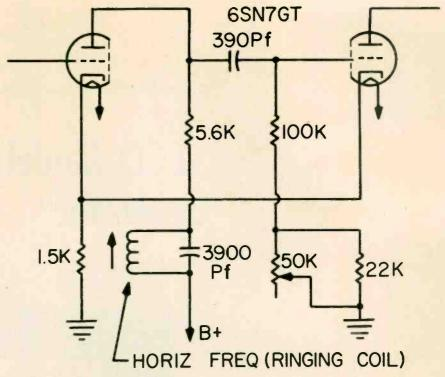
Fig. 4—Simplified circuit of horizontal oscillator using a ringing coil and 3900 pf capacitor.
