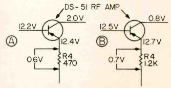
in later production is shown at "B." The result of this change is a minor increase in sensitivity which may not be noticeable. The important point is that the normal voltage readings differ somewhat.
