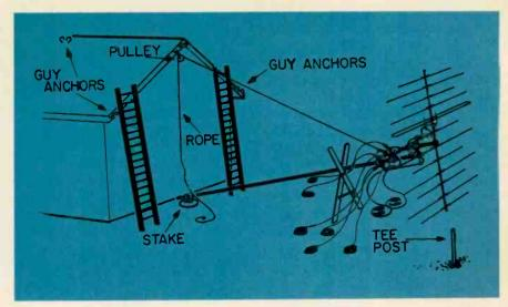
Fig. 1-Setup for erecting 40-ft antenna at end of house.
