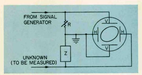
Fig. 2—Setup for high RF measurements when vertical amplifier response is not sufficiently high.
