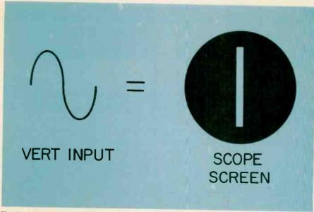
Fig. 3—A sinewave applied to the vertical plates will cause a straight vertical line on the CRT—if no sawtooth voltage is present on the horizontal plates.
