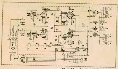
Fig. 1—Schematic of typical small stereo phono amplitier
