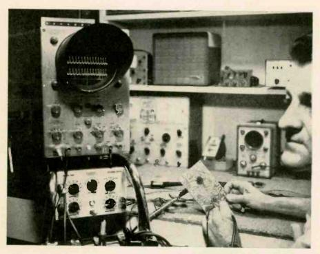
Technician testing a passive printed board removed from equipment.
