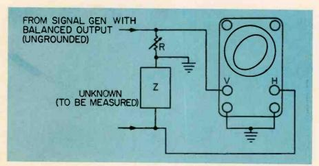
Fig. 1-Setup for making impedance measurements.
