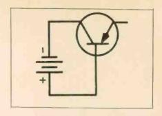
Is is not correct that  $I_{CO} = I_{CBO} =$ the reverse biased collector diode current with the emitter open-circuited, and would be measured as shown? ROBERT V. FLOYD
