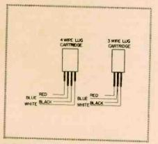
Fig. 2—Four wire and three wire stereo cartridges.
