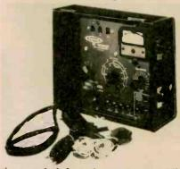
tions and defects is announced. The instrument also incorporates a voltmeter, capable of measuring up to 50,000 v. The meter has two voltage ranges—0 to 1000 and 0 to 50,000. The unit measures 9 x 12 x 5 in., and weighs 7.5 lb, according to the announcement. Amphenol.
