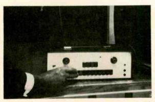
Jackson Model 800 Bar/Dot Generator NTSC type color signals. Patterns include cross-hatch, horizontal and vertical lines, dots and color bars. Gun killer. Has 14 tubes.
