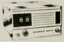
range the Courier 50 FM offers 50 w power coverage and is available with either ac or 12 vdc power ECI.
