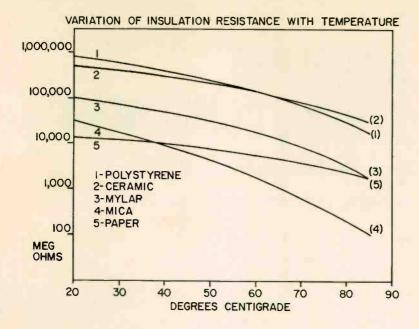
Fig. 2—Drift characteristics of popular capacitor materials.
