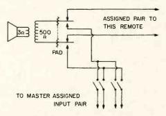
Fig. 7—Switches on remotes allow selection and contact with any master.
