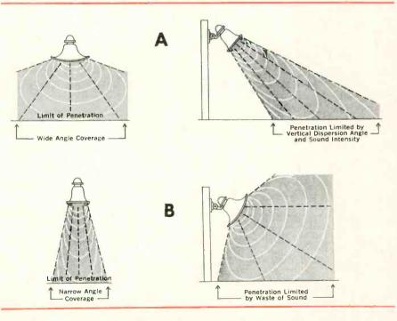
Fig. 1—Typical sound dispersion pattern of round directional horns. Angles range from 65 to 95 plane. (B)—Pattern of horn with long dimension in vertical plane.
