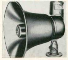
impedance taps, and 70.7 and 25 v power taps. HU15NT specifications are: Power, 25 w. Impedances, 45, 90, 180, 325, 670, 1000, 2000, 4000, 8000  $\Omega$ . 70.7 v line power taps, 15, 7.5, 2.5, 1.25, .65 w. 25 v line power taps, 14, 7, 3.5, 1.9, .92, .3 w. Frequency response 250-13,000 cps. Audio level, 123 db measured four ft on axis at rated power. Dispersion, 100 deg. Dimensions, 934 x 9 in. Write: Atlas Sound, 1419-51 39th St., Brooklyn, N. Y. 11218.
