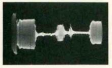
Fig. 2—The burst (center) with chroma information on both sides. The low frequency component has been removed at this point through capacitor coupling.
