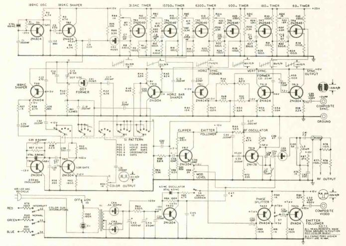
Fig. 2-Schematic of Sencore Model CG 135 Color Generator.
