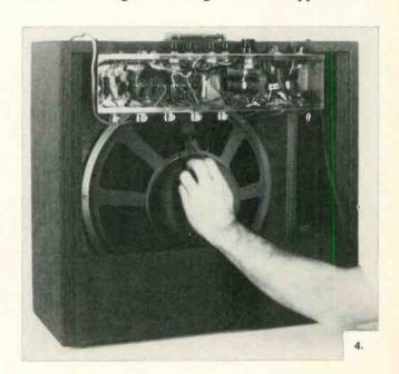
the same size, and can be more efficient in the midrange. (A speaker designed specifically for bass instruments will often have a copper voice coil since efficient reproduction of high frequencies is not required.)
