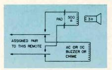
Fig. 2—Circuit used with one line pair and no monitoring remote.
