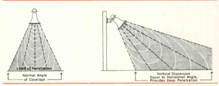
Fig. 1—Typical sound dispersion pattern of round directional horns. Angles range from 65 to 95 deg depending on horn size.
