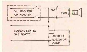
Fig. 5-Remote for more than one master and with call back feature.
