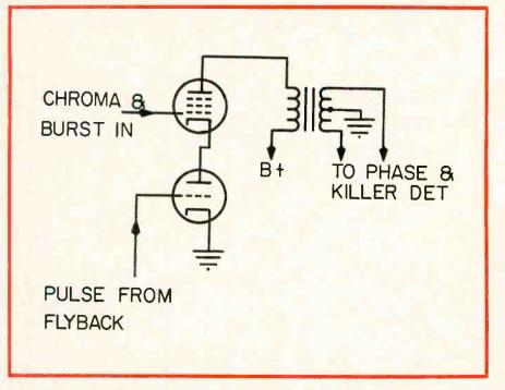
Fig. 6—Simplified schematic shows how gated burst amplifier is cut off by a pulse from the flyback—except when the burst is present—during retrace.
