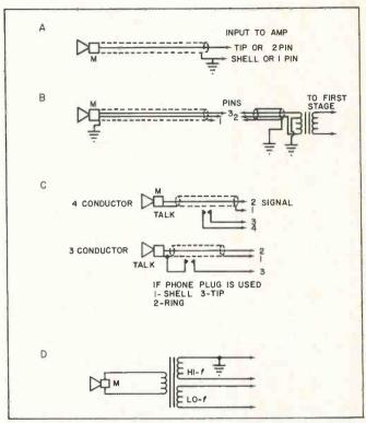
Fig. 3—(above) Common microphone connections. (A)—Single connector shielded. (B)—Two conductor shielded. (C)—Four and Three conductor push-to-talk circuits. (D)—Dual impedance microphone.
