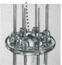
Stem assemblies are tested on a special highvacuum leak detecter. Detector is a helium mass-spectrometer, detecting passage of helium "tracer" gas through any of the glassto-metal seals. A stem assembly passing this rigorous test is ready to become a vital part of an RCA Silverama® Picture Tube.
