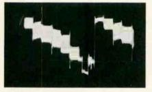
Fig. 1—. . . Scoot shouted, 'it looks like stair steps.' The bottom of the 'stair steps' is the horizontal sync pulse and immediately after it is the burst signal.
