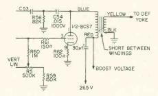
Shorted output transformer caused lack of vertical sweep.
