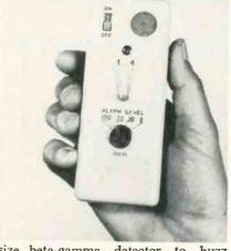
size beta-gamma detector to buzz when an alarm level of 3, 10, 30, or
