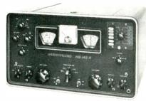
40, 20, 15, and 10 meter amateur bands; dual conversion above 10.0 Mc; six position crystal filter plus adjustable slot filter with up to 60 db attenuation; adjustable BFO for SSB and CW. A 1  $\mu$ v sensitivity gives 10:1 S/N ratio, the manufacturer says. Hammarlund.
