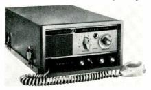
tal controlled channels is announced. In addition, the full broadcast band is available for listening to news, weather, and general programs. Transistorized audio amplifiers cut the receiver's battery drain to only 1.1 amp. Apelco.
