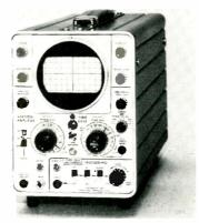
Mc, and maximum calibrated sensitivity is 10 mv/ $\frac{1}{4}$  in. div. A wide range time base provides calibrated sweep speeds to 0.5  $\mu$  sec/div; a X5 magnifier extends this sweep to approximately  $0.1\mu$  sec div. Tektronix.
