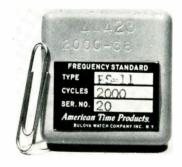
troduced. The output of type FS-11 is a limited sine wave of 3 v P-P min into  $30k \Omega$ . Standard input voltage is 28 vdc with units of lower input available. The unit is in a flat can  $1\frac{1}{2} \times 1\frac{1}{2} \times 3$ /8 in., with a 6 pin termination for circuit board applications. Operating temperature is -5 to  $85^{\circ}$  C and it weighs  $1\frac{1}{2}$  oz. Bulova.
