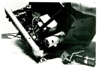
Fig. 6—Pencil points to topside-unit coils that were burned by lightning. Capacitor and selenium rectifier have been replaced.
