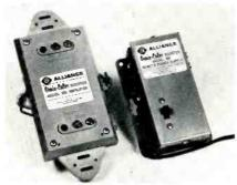
device combines an insertion gain of from 10 to 12 db, with a noise factor as low as 4 to 6 db, the manufacturer claims. The booster comprises a transistorized amplifier with universal mounting for any antenna boom or mast, or for wall or window frame installation. It is energized by a remote power supply unit which also functions as a two set coupler. Alliance.
