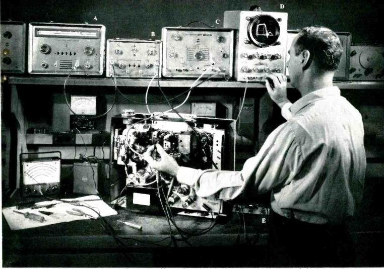
Checking overall frequency response (RF and IF) in a portable B&W TV receiver using the test instruments indicated in the block diagram below. Pattern on oscilloscope screen is an overall response curve with dual markers: one at picture-carrier frequency and one at sound-carrier frequency.
