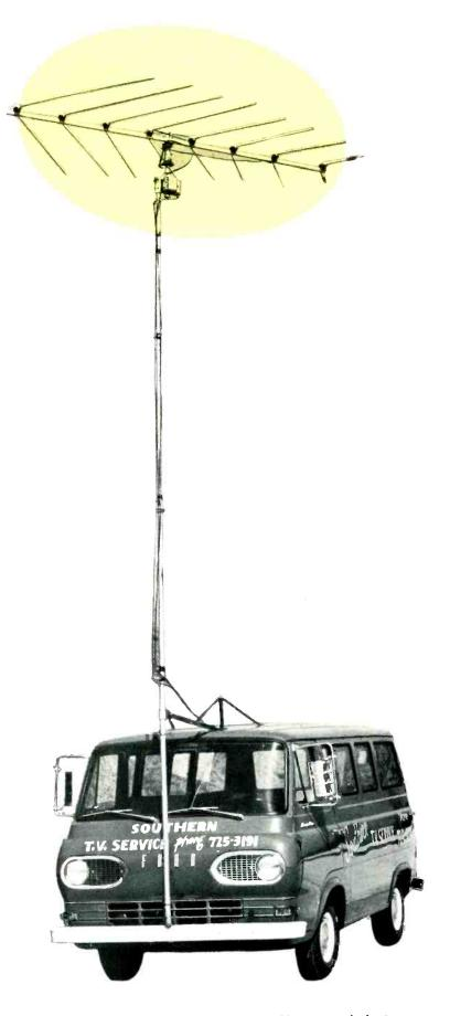
Motorized antenna elevated in receiving position on truck front
