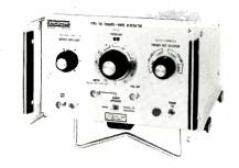
erator with nanosec rise and fall times and extremely wide operational frequency range is announced. Termed the Fairchild type 791, the solid-state generator provides performance characteristics not previously available in one instrument, the announcement revealed. Rise and fall times of the square waves are kept constant throughout all frequencies from 7 cps to 10 Mc the maker said. Fairchild.
