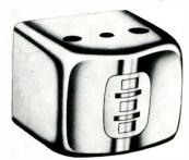
contour which meets NAB standards for tape cartridge players in stereo applications. Designed for three-channel record and playback, this head has three 0.043-in. tracks located on 0.100-in. centers, deposited quartz gaps and precision lapped, low-loss core structures, the announcement said. Available in rear-mount, base-mount, side-mount and no-mount styles. Nortronics.
