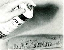
Liquid rubbers permit encapsulation of circuitry by the spray method.
