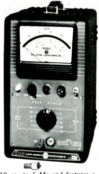
10 cps to 6 Mc and features a 1 percent accuracy fsd from 40 cps to 1 Mc. Ballantine.
