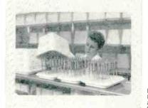
Electron guns, after drying, are kept in covered racks as further assurance against dust contamination.
